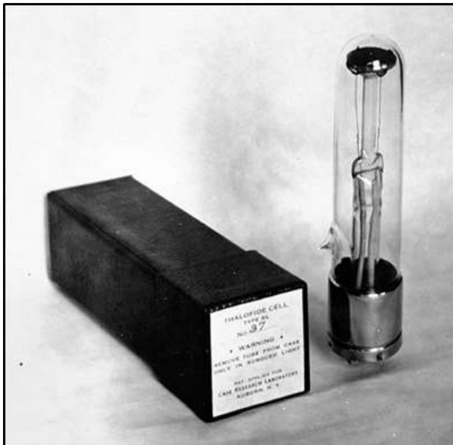
Figure 3: Thalofide cell packaging, with cell (10cm in height approx.) on the right. Courtesy of the Cayuga Museum and Case Research Lab.
