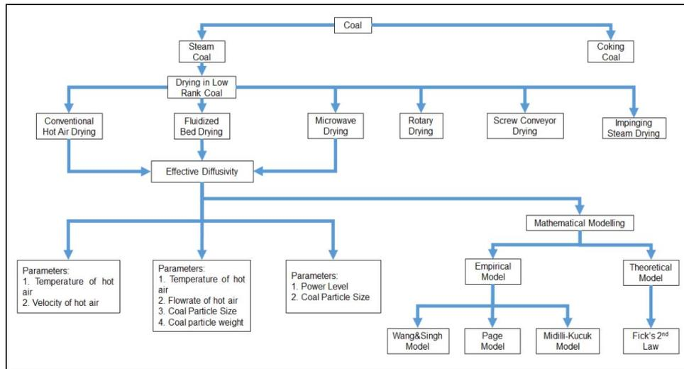
**Figure 2.** Diffusivity in drying of low rank coal
