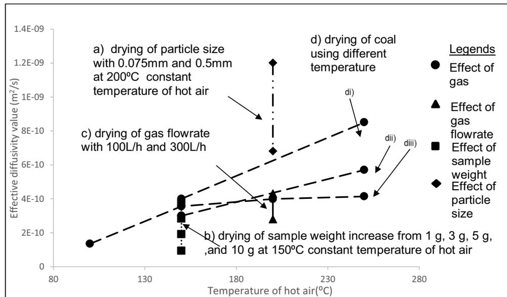
**Figure 5.** A plot of temperature of hot air versus effective diffusivity using fluidised bed drying. (a) drying of particle size (b) drying of sample weight (c) drying of gas flowrate (d) drying of coal using different temperature
