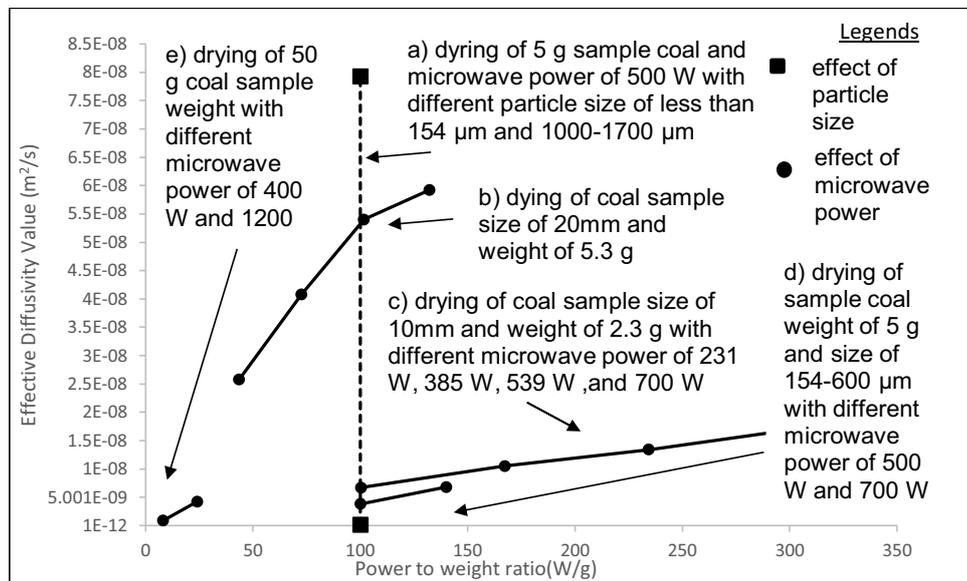
**Figure 6.** Power to weight ratio versus effective diffusivity value. (a) drying with different particle size (b) drying with different microwave power (c) drying with different microwave power (d) drying with different microwave power (e) drying with different microwave power
