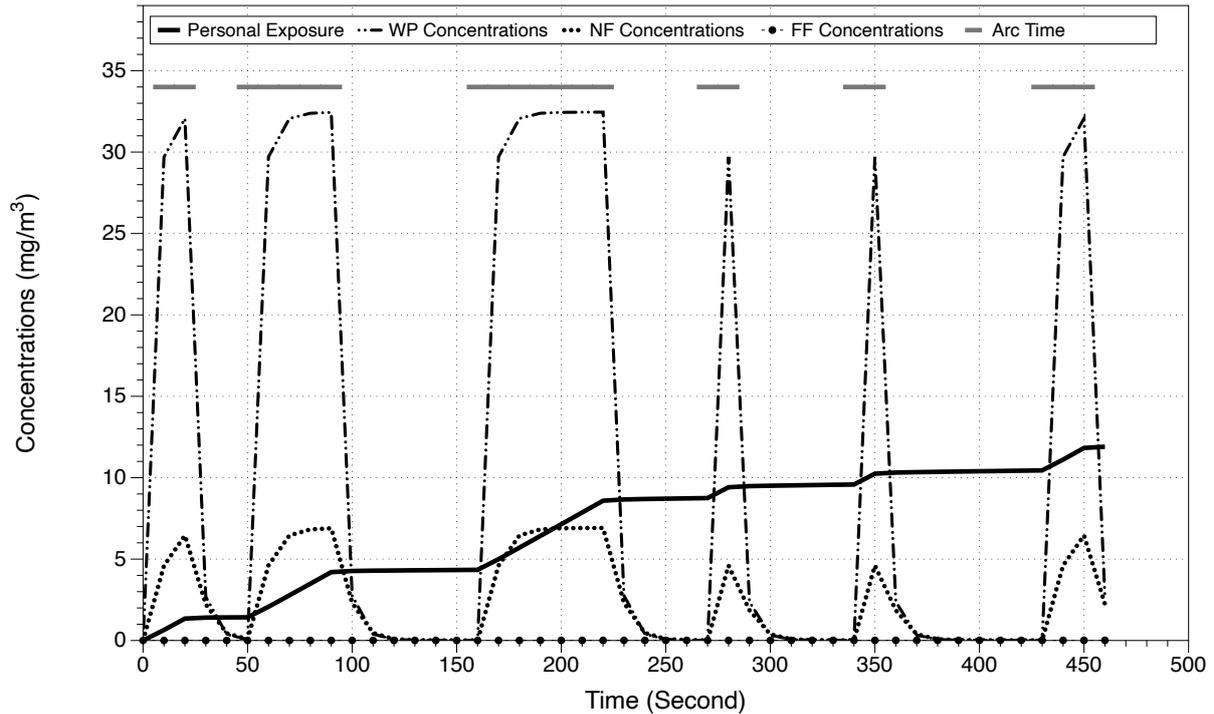
**Fig. 5.** The example (Sample ID 2) of the pattern of welding fume concentrations in the different compartments.
