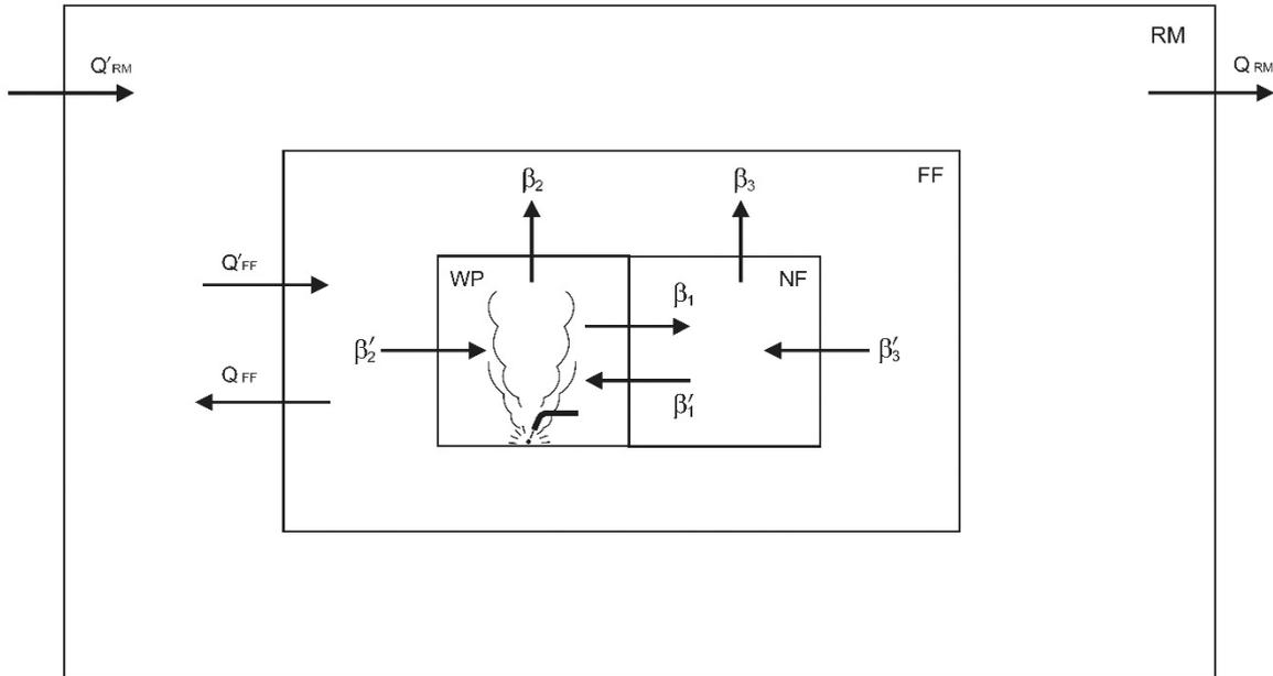
**Fig. 2.** A conceptual diagram of the weldART model with four compartments.
