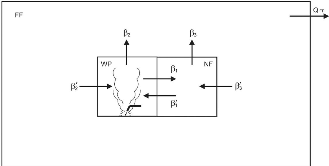
**Fig. 1.** A conceptual diagram of the weldART model with three compartments.
