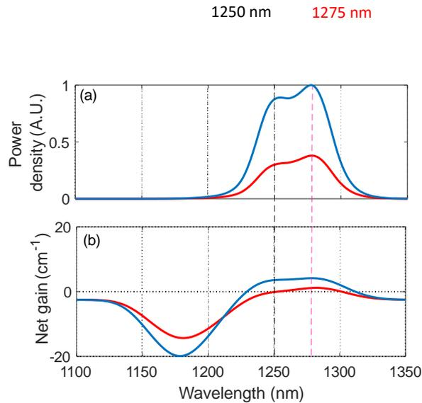
Fig. 6. Simulation results for a rear section current of  $0.17 \text{ kAcm}^{-2}$  and a front section current of  $0.3 \text{ kAcm}^{-2}$ . (a) Rear (red line) and front (blue line) output power spectra. (b) Net gain in  $z=0$  (red line) and in  $z=L$  (blue line).
