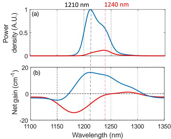
Fig. 7. Simulation results for a rear section current of  $0.17 \text{ kAcm}^{-2}$  and a front section current of  $1 \text{ kAcm}^{-2}$ . (a) Rear (red line) and front (blue line) output power spectra. (b) Net gain in  $z=0$  (red line) and in  $z=L$  (blue line).
