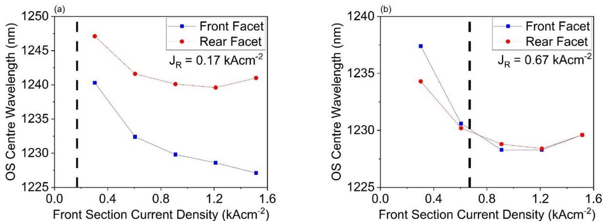
Figure 3. Plots of front and rear facet optical spectra (OS) center wavelength vs front section current density at a fixed rear section current density ( $J_R$ ) of  $0.17 \text{ kAcm}^{-2}$  (a) and  $0.67 \text{ kAcm}^{-2}$  (b). Black dashed lines mark the point where the front and rear section current densities were equal.
