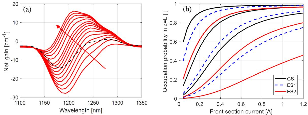
Fig. 5. (a) Average net gain in  $z=0$  (black dashed line) and  $z=L$  (red continuous lines). The current in the rear section is  $0.17 \text{ kAcm}^{-2}$ , while the current in the front section is changed from  $0.04 \text{ kAcm}^{-2}$  to  $1.2 \text{ kAcm}^{-2}$ . (b) Occupation probability in the GS, ES1, and ES2 confined states of the three type of chirped QD layers, for a  $0.17 \text{ kAcm}^{-2}$  rear section current.
