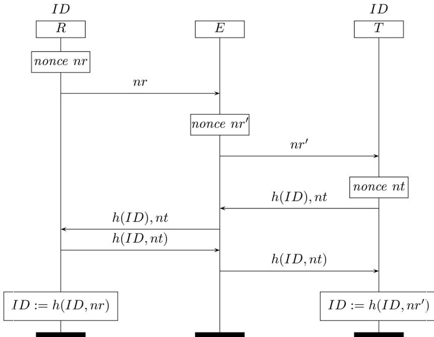
Fig. 2. Desynchronization attack on the HMNB protocol
