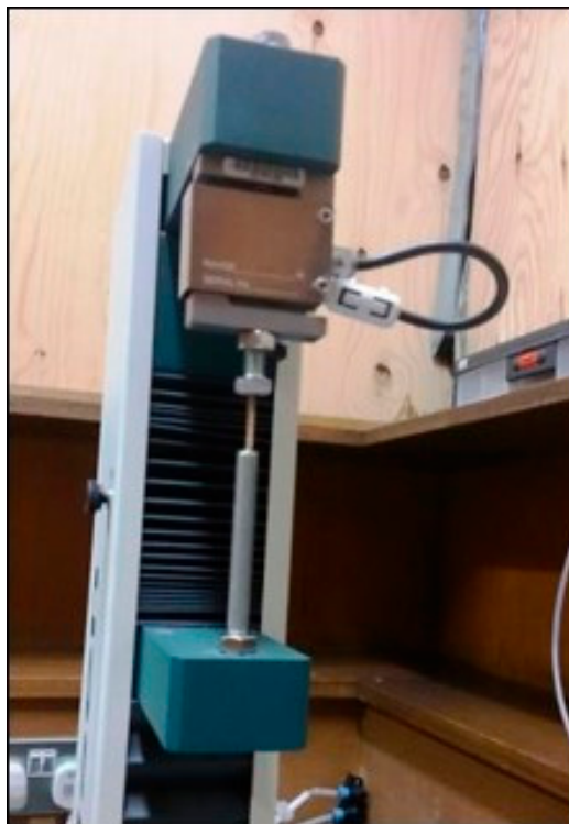
Figure 2. Compressive testing apparatus, recording the deformation curve of a historic sample of pine. This allows the calculation of the modulus of elasticity of the sample to be calculated.
