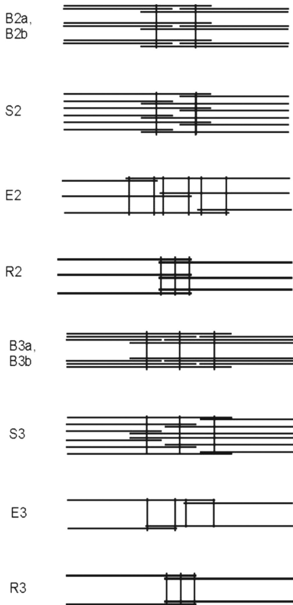
Fig. 4—Main reinforcement splice details (not to scale).
