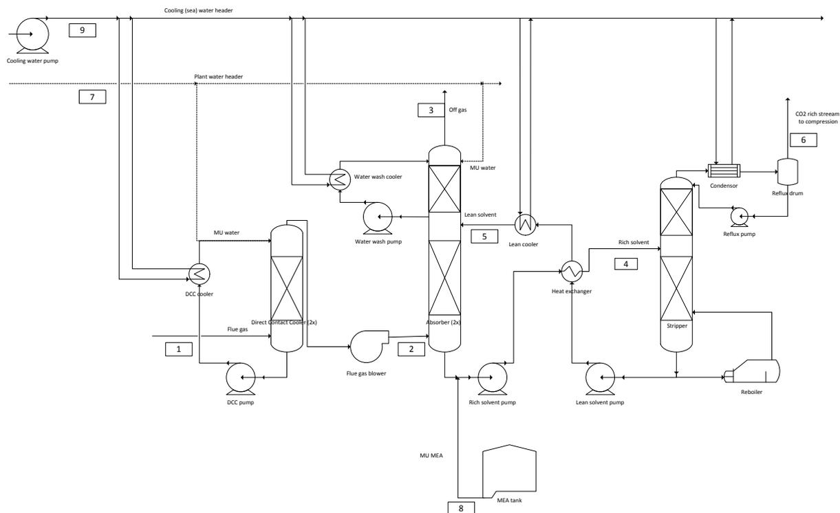
Figure 3. Process Flow Diagram of the MEA model.
