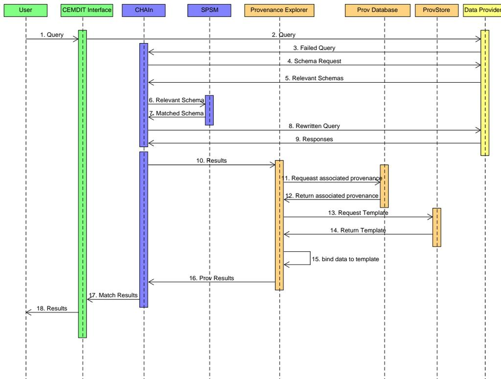
Figure 1. Sequence diagram showing the flow of data in the CEM-DIT system
