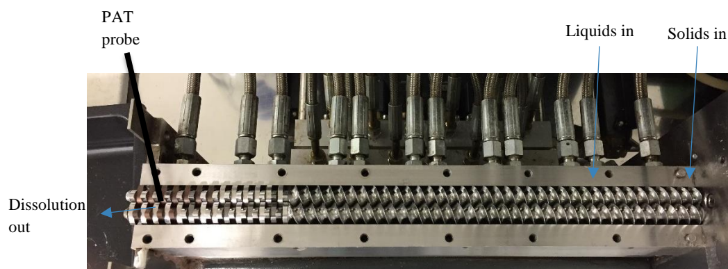
Figure 5 Twin screws inside barrel of continuous twin screw extruder
