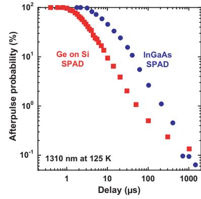
Fig. 3. The afterpulsing for a 100  $\mu\text{m}$  diameter Ge-on-Si SPAD compared to a 26  $\mu\text{m}$  diameter InGaAs/InP SPAD under nominally identical conditions ( $T = 125 \text{ K}$  and 17% SPDE at 1310 nm).
