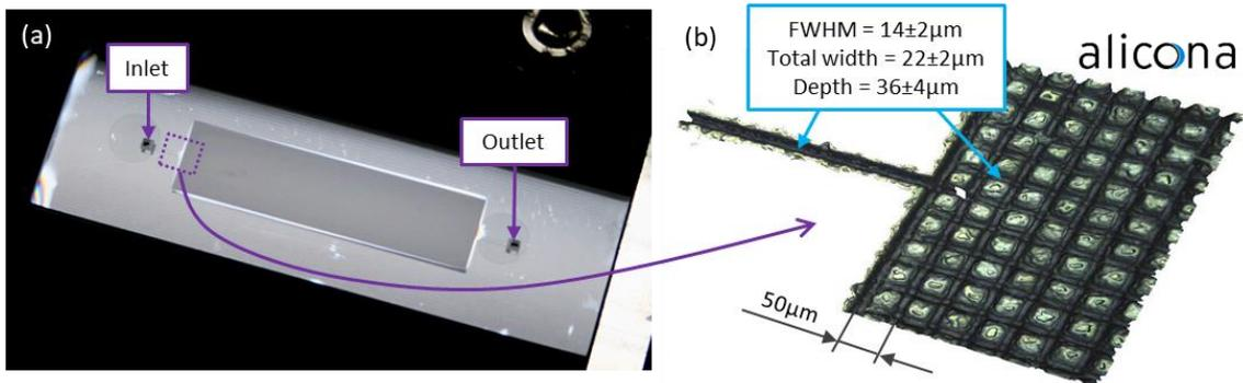
Figure 1: Enclosed microfluidic device manufactured using a picosecond laser: (a) photograph and (b) 3D surface profile of microchannels.
