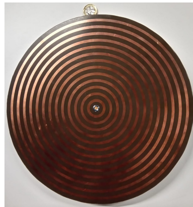
Fig. 1. Fabricated and measured planar leaky-wave antenna. Copper color: annular metallic strip arrangement. Dark color: grounded dielectric slab. The structure is made by a slot grating on a grounded dielectric slab (GDS). Strips having width w = 1 mm and period d = 8 mm define the top PRS. The GDS is made by a dielectric with \epsilon_r = 2.2 and thickness h = 3.14 mm.
