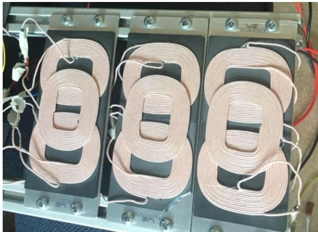
Fig. 11. The  $3 \times 3$  coil array structure.
