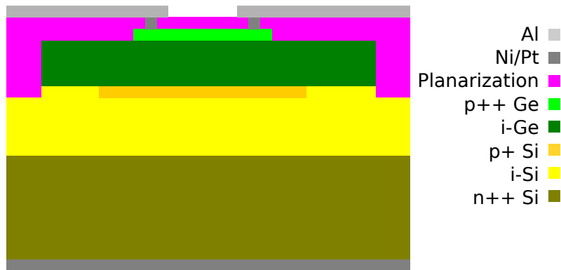
Figure 2. The structure of the device is composed of an n ++ Si substrate, with a 1.5 \mu\text{m} i-Si multiplication region with implanted charge sheet at the top. Followed by an epitaxially grown 1 \mu\text{m} i-Ge absorption layer, and 50 \text{ nm} p ++ Ge top contact layer.
