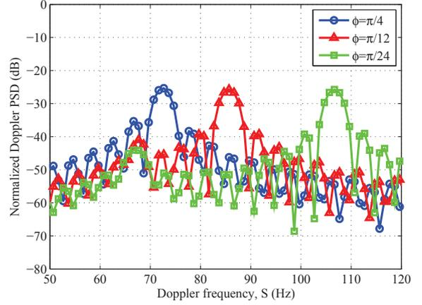
Fig. 5. Normalized Doppler PSDs of different communication elevation angles.
