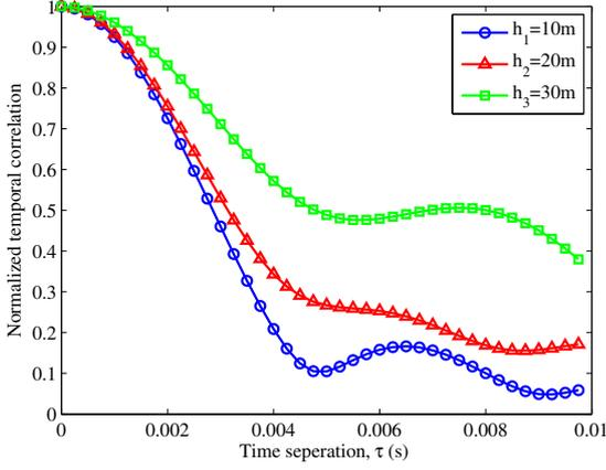
Fig. 3. Temporal ACFs of different UAV altitudes.
