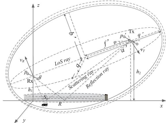
Fig. 1. A 3D GBSM for A2G channels.
