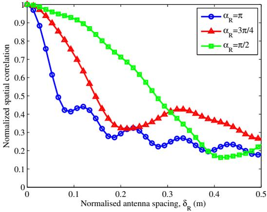
Fig. 4. Spatial CCFs at TX side for different antenna orientation.
