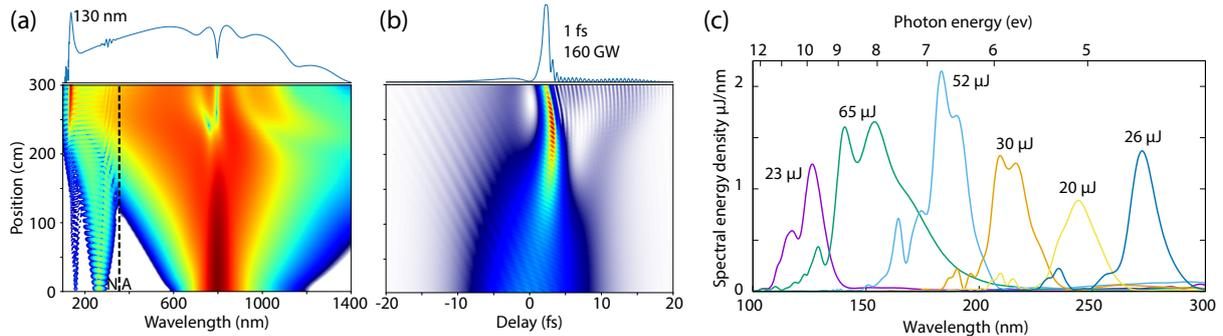
**Fig. 1:** Numerically modelled spectral (a) and temporal (b) evolution of a 10 fs, 800 nm, 0.5 mJ pump pulse in a 250  $\mu\text{m}$  inner diameter HCF filled with 0.3 bar He. N, A indicate normal and anomalous dispersion regions. (c) Optimized VUV dispersive-wave emission peaks, for different He gas pressures.
