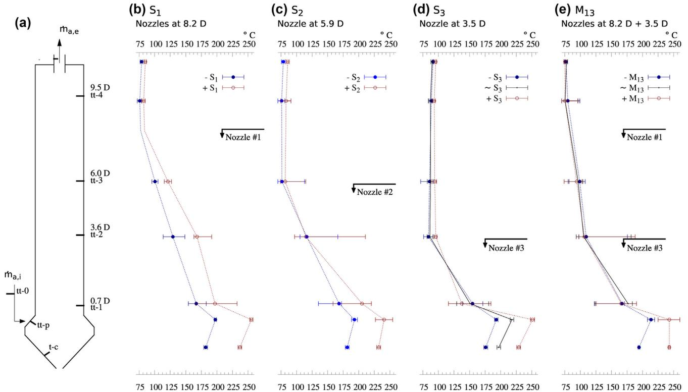
Fig. 5. Cross-sectional average  $T_{A,av}$  from tt-1 to tt-4, time averaged  $T_A$  measurements in tt-p and single punctual  $T_A$  measurements in t-c. (a) Location of sensors, (b) operation of nozzle #1 at 8.2 D, (c) operation of nozzle #2 at 5.9 D, (d) operation of nozzle #3 at 3.5 D, and (e) operation from nozzles #1 and #3.
