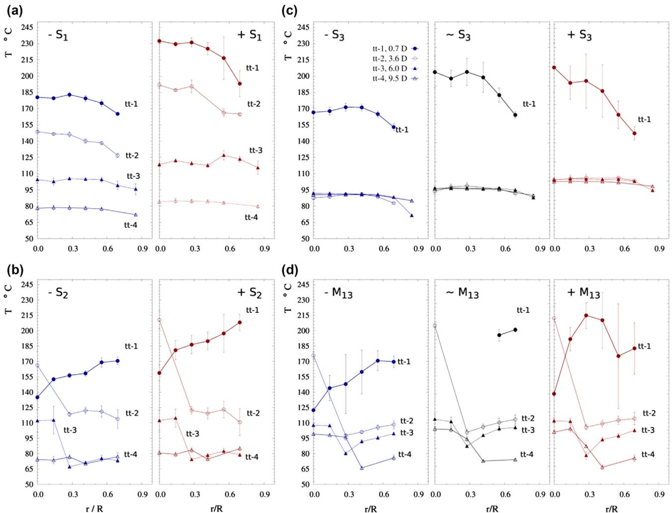
**Fig. 4.** Time averaged air temperature  $T_A$  radial profiles for tt-1 at 0.7 D, tt-2 at 3.6 D, tt-3 at 6.0 D, tt-4 at 9.5 D. (a) Operation of nozzle #1 at 8.2 D, (b) operation of nozzle #2 at 5.9 D, (c) operation of nozzle #3 at 3.5 D, and (d) operation from nozzles #1 and #3.
