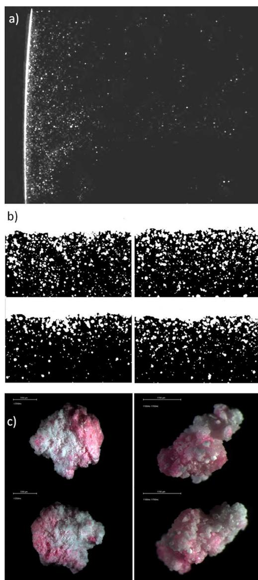
**Fig. 1.** Visualization of the wall dynamics: (a) and (b) show the near wall region and multi-layered deposits observed under Particle Image Velocimetry, PIV, reproduced from Hassall (2011). (c) Granules  $>850$  during  $S_2$  whereby the colour tracer tracks material resuspended from the deposits (Francia et al., 2015a). (For interpretation of the references to colour in this figure legend, the reader is referred to the web version of this article.)
