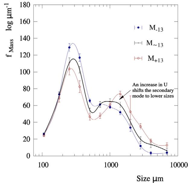
**Fig. 12.** Variation of the product size using two spraying levels from the reference case  $M_{-13}$  (black) (Francia et al., 2016b) to a hot weak vortex ( $\uparrow T_A \downarrow U_A^2$  in  $M_{+13}$  (+, red) or a cold strong vortex ( $\downarrow T_A \uparrow U_A^2$  in  $M_{-13}$  (–, blue). (For interpretation of the references to colour in this figure legend, the reader is referred to the web version of this article.)
