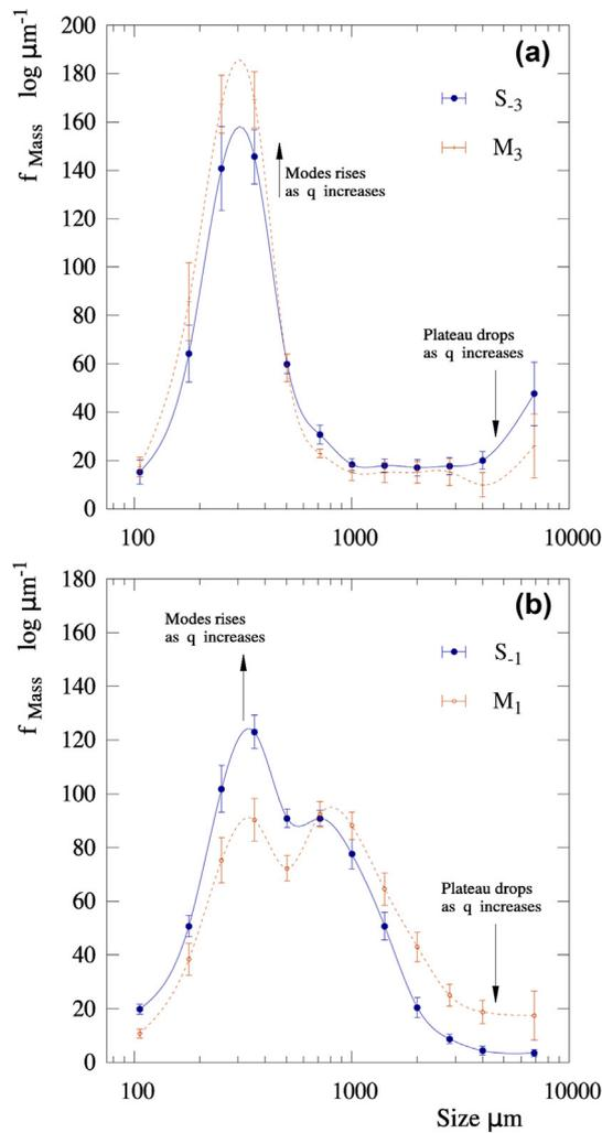
**Fig. 13.** Comparison of the product size resulting from nozzles #1 and #3 in multi-level operation conditions,  $M_1$  and  $M_3$  (Francia et al., 2016b) to under a cold strong vortex  $\downarrow T_A \uparrow U_A^2$  (–, blue),  $S_{-1}$  and  $S_{-3}$ . (a) Bottom nozzle #3,  $M_3$  and  $S_3$ , (b) top nozzle #1,  $M_1$  and  $S_1$ . (For interpretation of the references to colour in this figure legend, the reader is referred to the web version of this article.)
