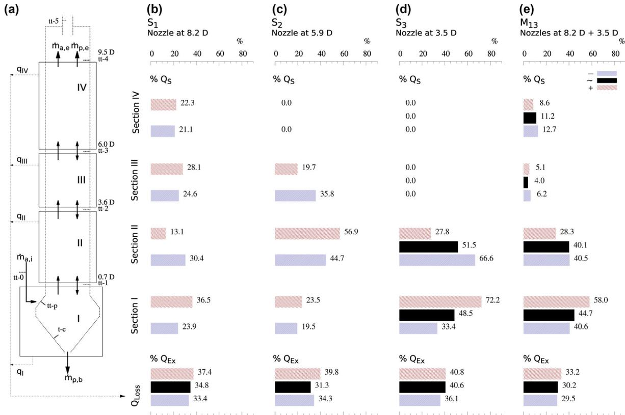
**Fig. 6.** (a) Definition of Section I, Section II (containing nozzle #3), Section III (containing nozzle #2) and Section IV (containing nozzle #1). Heat losses,  $Q_{Loss}$ , and distribution of the rate of heat transferred to the solids,  $Q_s$  (b)  $S_1$ , nozzle at 8.2 D (c)  $S_2$ , nozzle at 5.9 D (d)  $S_3$ , nozzle at 3.5 D, (e)  $M_{13}$ , nozzles at 8.2 D and 3.5 D.
