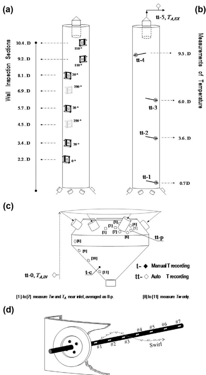
Fig. 3. Measurements: (a) wall inspection areas, (b) air temperature,  $T_A$  sensors in the cylinder and exhaust line, (c)  $T_A$  sensors at inlet, bottom sections and at the walls,  $T_w$ , and (d) arrangement of thermocouples inside hollow bars.
