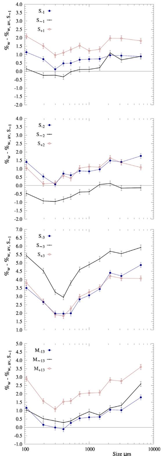
**Fig. 14.** Product water content  $X_w$ . (a)  $S_1$ , (b)  $S_2$ , (c)  $S_3$  and (d)  $M_{13}$ . Comparison of reference productions ( $\sim$ , Francia et al., 2016a, 2016b black) to a hot weak vortex  $\uparrow T_A \downarrow U_A^2$  (+, red) and a cold strong vortex  $\downarrow T_A \uparrow U_A^2$  (–, blue). (For interpretation of the references to colour in this figure legend, the reader is referred to the web version of this article.)
