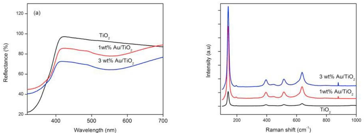
Figure 3. a) Diffuse reflectance spectra and b) Raman spectra of pure TiO<sub>2</sub> and Au/TiO<sub>2</sub> samples.
