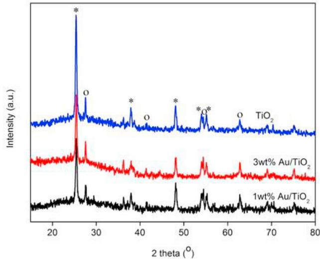
Figure 2. XRD pattern of pure TiO<sub>2</sub> anatase (\*) and rutile (o) and Au/TiO<sub>2</sub> samples.
