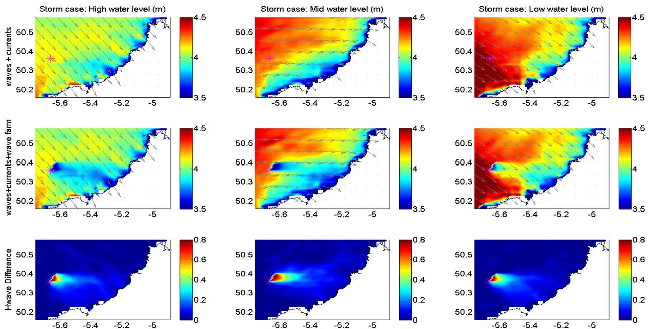
Fig. 5 Significant wave height (colours) and wave direction (vectors) for the storm case and for the tidal cycle cases. In this figure is shown the difference (bottom panels) between the wave-current interaction (top panels) and the wave-current & wave farm interaction (middle panels). Wave Hub site (\*).
