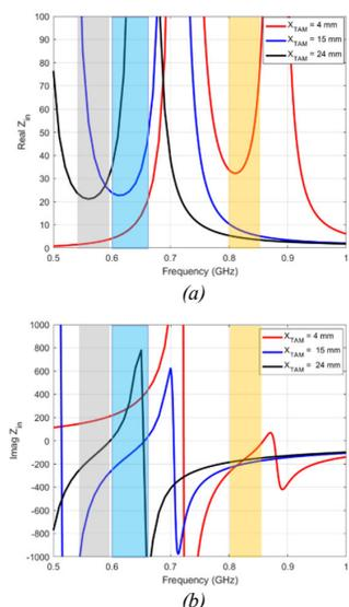
Fig. 3 Input impedance of the CPW-fed three-arm dipole  $X_{TAM}$ : real part (a), imaginary part (b).
