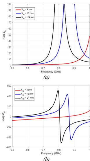
Fig. 2 Input impedance of the CPW-fed monopole antenna as a function of parameter  $X_M$ : real part (a), imaginary part (b).
