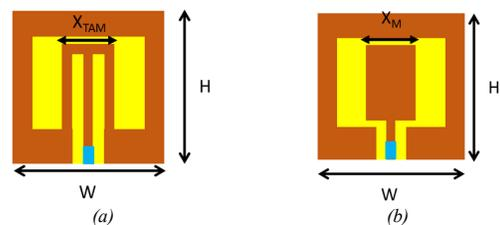
Fig. 1 Investigated CPW-fed antennas: (a) Three-arm dipole and (b) monopole. The blue rectangle represents the input port.
