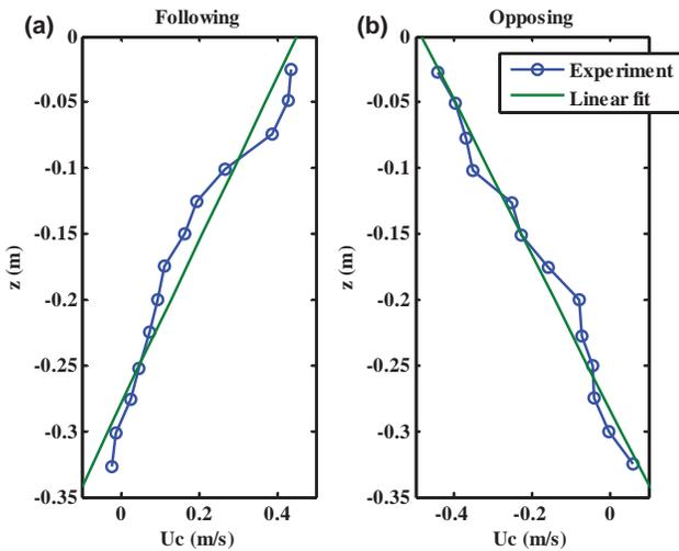
Fig. 2 Measured shear current profiles in Swan (1990). (a) case 2F: linearly sheared following current; (b) case 2A: linearly sheared opposing current.
