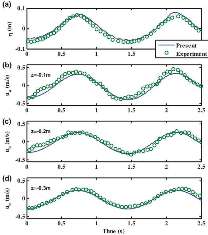
Fig. 5 Predicted (-) and observed (o) surface elevation (a) and horizontal wave velocities (b)-(d) under linearly sheared opposing current (case 2A).
