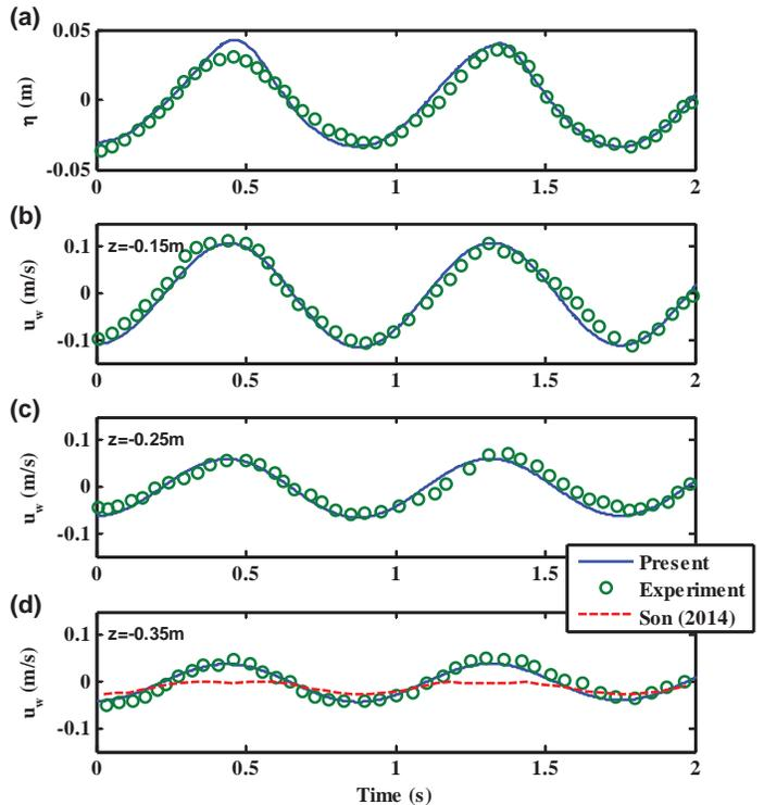
Fig. 4 Predicted (-) and observed (o) surface elevation (a) and horizontal wave velocities (b)-(d) under uniform, following current (case 1A).
