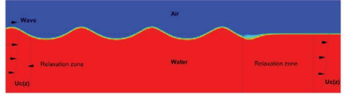
Fig. 1 Schematic of the 2D numerical wave-current flume
