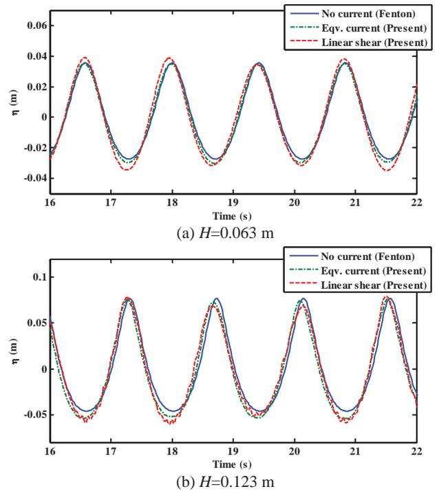
Fig. 7 Current shear effect on water surface elevations (opposing current). Solid: analytical no current, wave-only solution (Fenton, 1985); dash-dot: prediction with equivalent uniform current; dashed: prediction with linearly sheared current.
