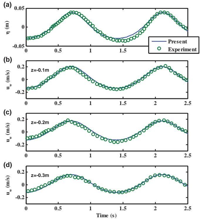
Fig. 3 Predicted (-) and observed (o) surface elevation (a) and horizontal wave velocities (b)-(d) under uniform, following current (case 1F).
