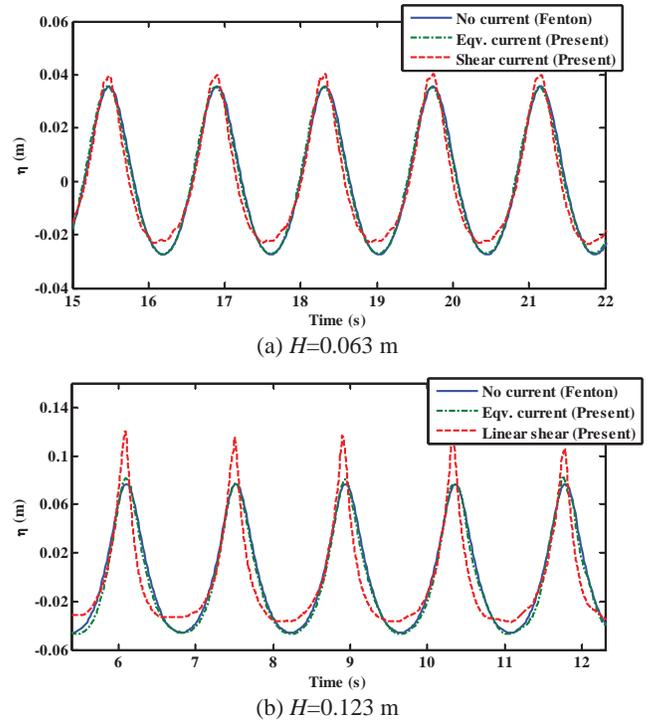
Fig. 6 Current shear effect on water surface elevations (following current). Solid: analytical no current, wave-only solution (Fenton, 1985); dash-dot: prediction with equivalent uniform current; dashed: prediction with linearly sheared current.
