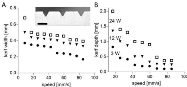
**Figure 3.** (A) Influence of laser power and speed on the kerf width (B) kerf depth. In insert a cross section picture of a channel engraved with a power of 12 W and a speed of 15 mm/s. scale bar is 500  $\mu\text{m}$ .
