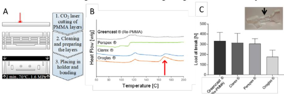
**Figure 1.** A) Overview of PMMA rapid-prototyping technique described in [4]. We propose a sustainable alternative by replacing pristine PMMA by Re-PMMA B) Thermograms of the Re-PMMA, Perspex®, Clarex® and Oroglas®; C) Maximum bonding strength of Re-PMMA, Clarex®, Perspex® and Oroglas®; In Inset, Photograph of the broken specimen (Re-PMMA). The black arrow points where the material break, showing the other part of the specimen still bonded.
