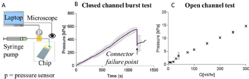
**Figure 2.** A) Experimental set-up; B) Burst test in close channels (width 250  $\mu\text{m}$ ). Maximum pressure difference in function of flow rate. Deviation is shown in grey; C) Open channel tests. Input flow rate in function of pressure. 300mL/h was the pump maximum flow rate. For some points the error bar is shorter than the symbol.
