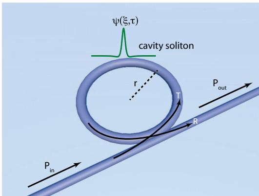
FIG. 1 (color online). Sketch of the generic microcavity and its parameters.  $r$  is the ring radius,  $P_{\text{in}}$  is the cw input power,  $P_{\text{out}}$  is the output field power,  $\psi(\xi, \tau)$  is the intracavity field at position  $\xi$  in the ring, and  $R$  and  $T$  are the reflection and transmission coefficients, respectively.
