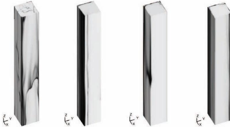
**Figure 2:** Instantaneous particle volume fraction field in the periodic circulating fluidized bed for different mesh resolutions. From right to left, the mesh resolution increases. White color corresponds to  $\alpha_p = 0$ . Black color corresponds to  $\alpha_{p,max} = 0.64$ .
