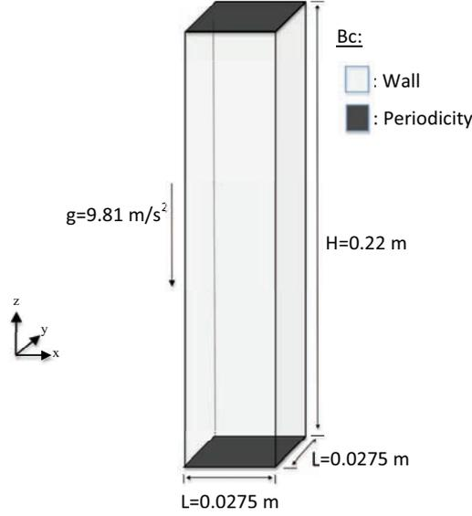
**Figure 1:** The periodic circulating fluidized bed (PCFB).
