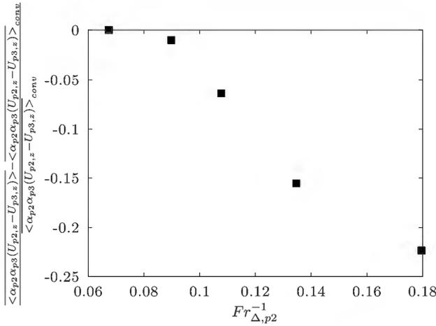
**Figure 5:** Influence of the mesh size, based on the smaller particle inverse Froude number, on the inter-particle relative velocity  $\overline{\alpha_{p2}\alpha_{p3}(U_{p2,z} - U_{p3,z})}$ . The subscript *conv* corresponds to the converged case,  $Fr_{\Delta,p2}^{-1} = 0.064$ .
