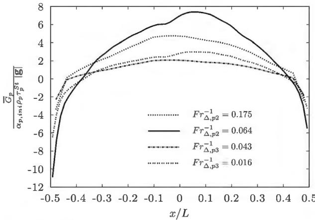
**Figure 9:** Radial profile of time-averaged total vertical solid mass flux of the particulate phases  $\bar{G}_{p2}$  and  $\bar{G}_{p3}$  for two mesh resolutions: coarse ( $24 \times 24 \times 192$ ,  $Fr_{\Delta,p2}^{-1} = 0.175$  and  $Fr_{\Delta,p3}^{-1} = 0.043$ ), fine ( $64 \times 64 \times 512$ ,  $Fr_{\Delta,p2}^{-1} = 0.043$  and  $Fr_{\Delta,p3}^{-1} = 0.016$ ).
