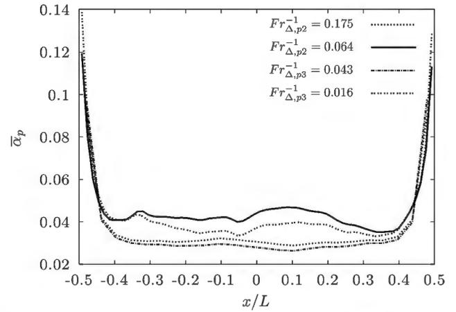
**Figure 7:** Radial profile of time-averaged solid volume fraction of the particulate phases  $\alpha_{p2}$  and  $\alpha_{p3}$  for two mesh resolutions: coarse ( $24 \times 24 \times 192$ ,  $Fr_{\Delta,p2}^{-1} = 0.175$  and  $Fr_{\Delta,p3}^{-1} = 0.043$ ), fine ( $64 \times 64 \times 512$ ,  $Fr_{\Delta,p2}^{-1} = 0.043$  and  $Fr_{\Delta,p3}^{-1} = 0.016$ ).
