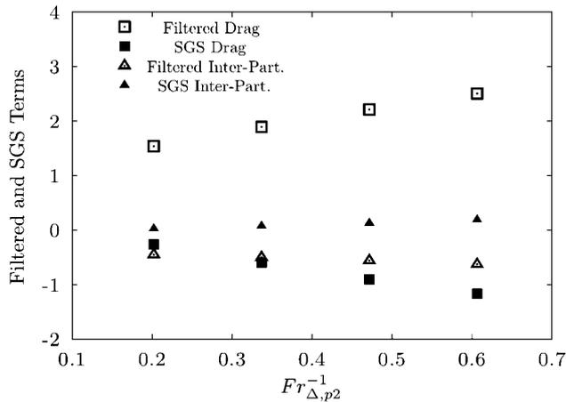
**Figure 11:** Filtered and sub-grid contributions drag and inter-particle collision forces normalised by the gravity term with respect to different inverse Froude numbers based on the filter width  $\bar{\Delta}$  for small particles (75  $\mu\text{m}$ ).
