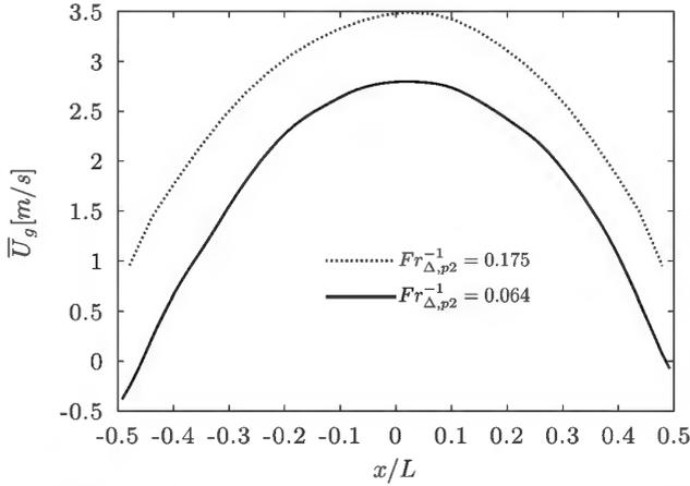
**Figure 8:** Radial profile of time-averaged vertical gas velocity for two mesh resolutions: coarse ( $24 \times 24 \times 192$ ,  $Fr_{\Delta,p2}^{-1} = 0.175$  and  $Fr_{\Delta,p3}^{-1} = 0.043$ ), fine ( $64 \times 64 \times 512$ ,  $Fr_{\Delta,p2}^{-1} = 0.043$  and  $Fr_{\Delta,p3}^{-1} = 0.016$ ).
