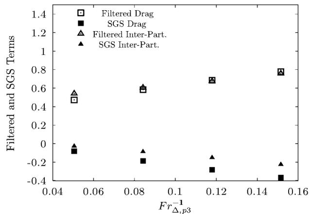
**Figure 12:** Filtered and sub-grid contributions drag and inter-particle collision forces normalised by the gravity term with respect to different inverse Froude numbers based on the filter width  $\bar{\Delta}$  for large particles (150  $\mu\text{m}$ ).
