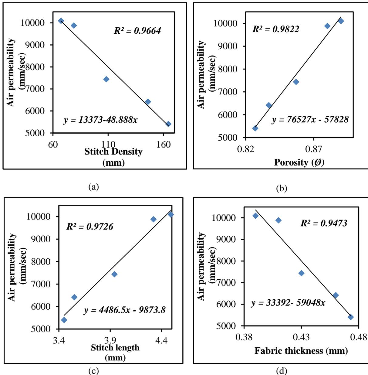
**Figure 6.** Relationship between predicted air permeability and (a) stitch density, (b) porosity, (c) stitch length, and (d) fabric thickness
