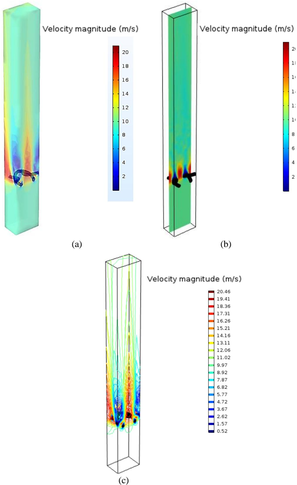
**Figure 5.** Simulated results of plain weft knitted fabric F2: (a) Magnitude of the velocity field in the free and porous plain weft knitted domains, (b) Slice view of velocity magnitude and (c) Contour of velocity magnitude
