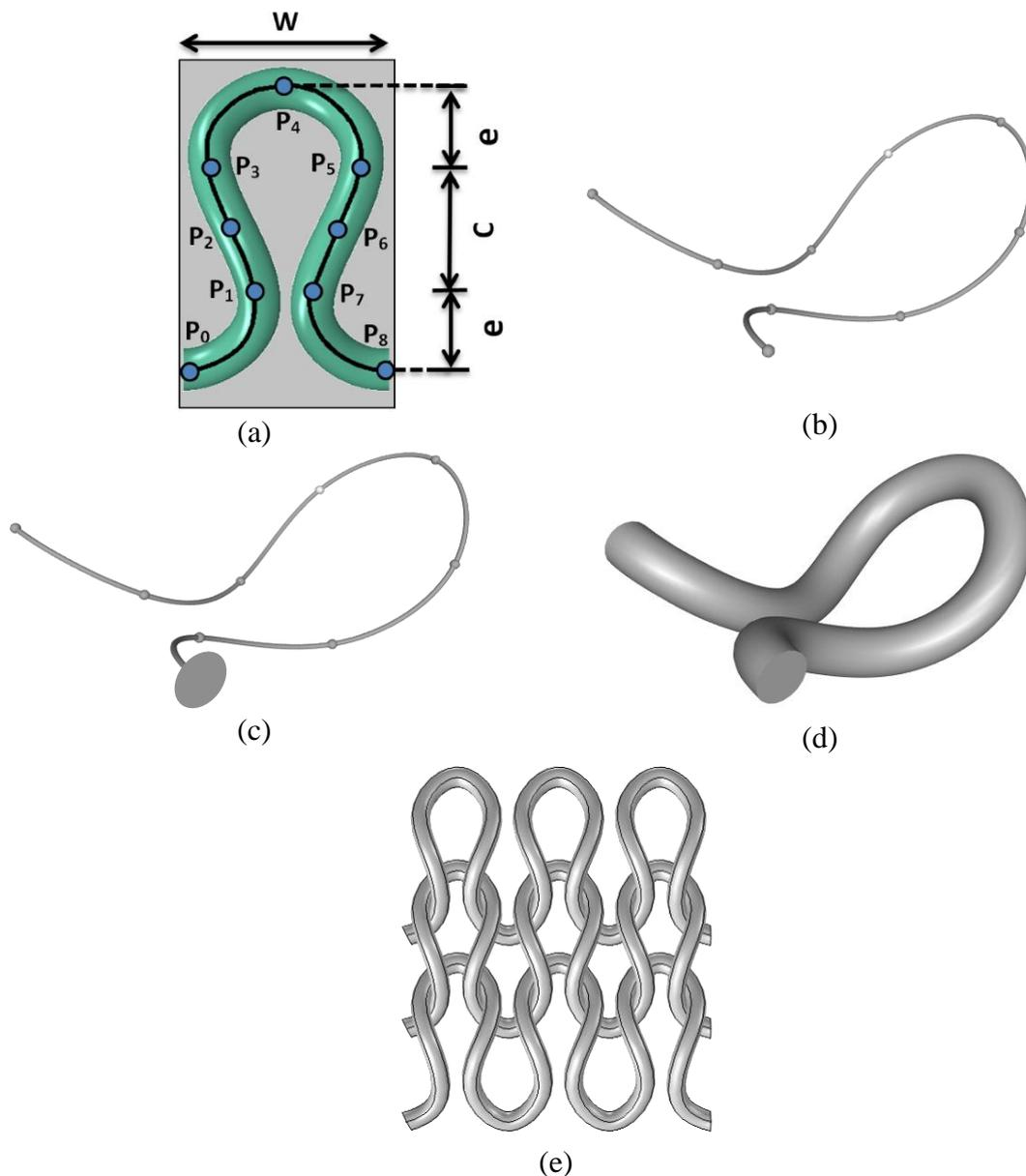
**Figure 2.** 3D model of plain knitted fabric: (a) Geometry of a plain weft knitted loop (11), (b) Yarn path or central axis, (c) Yarn path with circular cross-section, (d) 3D loop of knitted fabric, (e) Geometrical model of fabric F5
