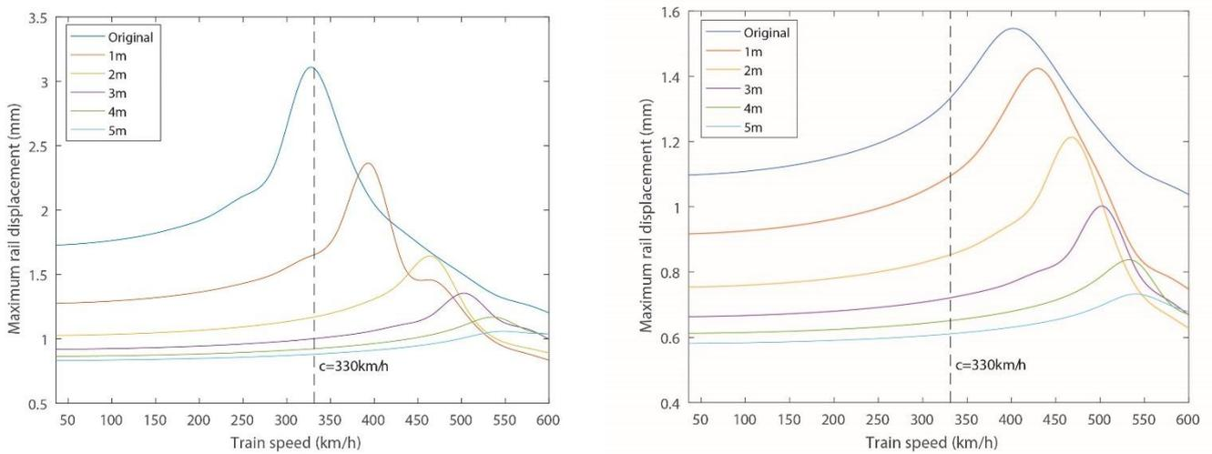
Figure 20: Maximum vertical rail displacement vs train speed, for Soil 2 with different depths of soil replacement strategies. (Left) Ballasted track; (Right) Slab track
