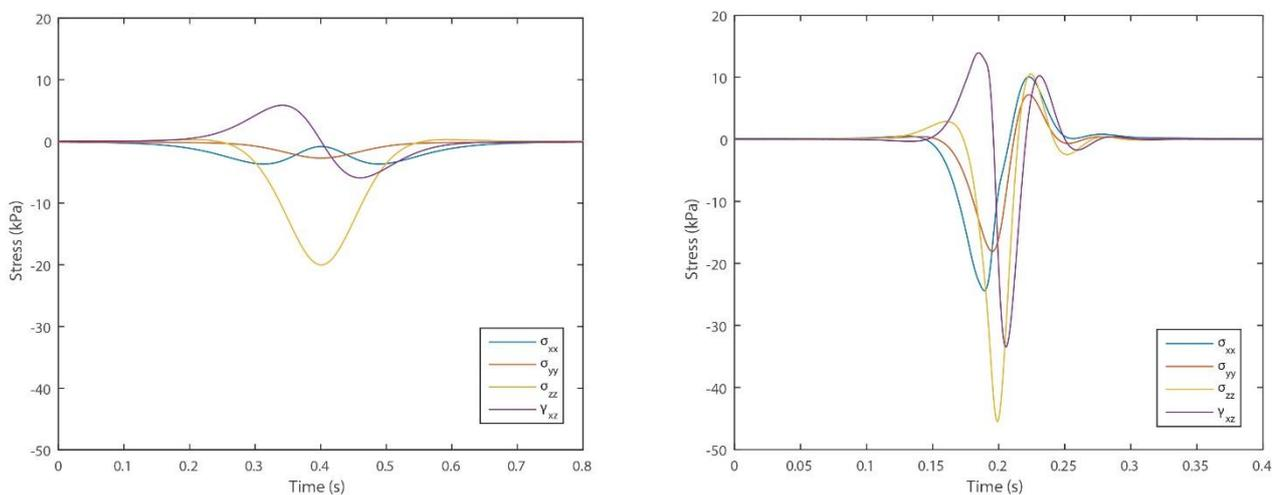
Figure 17: Stress time history comparison at the surface for ballasted track. (Left)  $c=20\text{m/s}$  (Right)  $c=92\text{m/s}$
