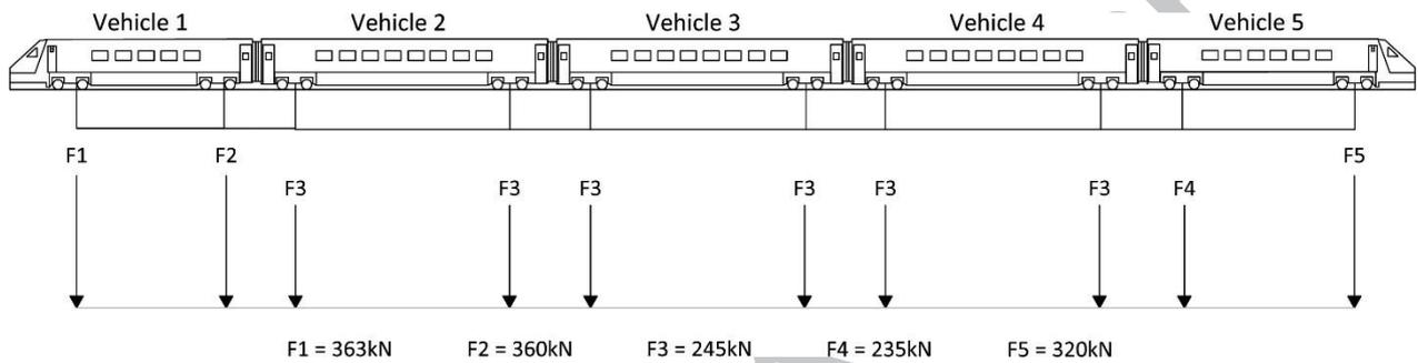
Figure 8: Train loads applied in the numerical simulation
