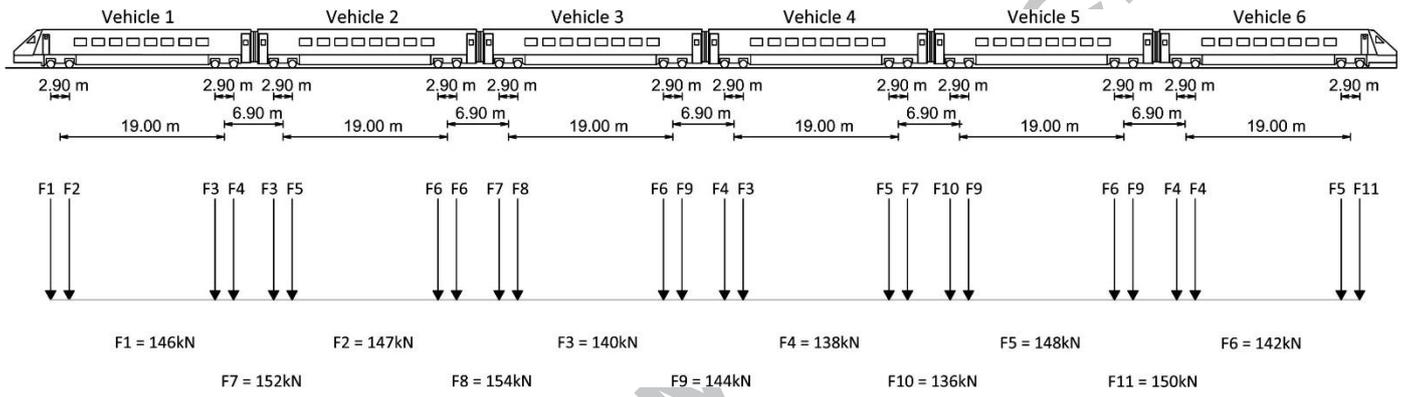
Figure 12: Geometry and mechanical properties of the Alfa-Pendular train
