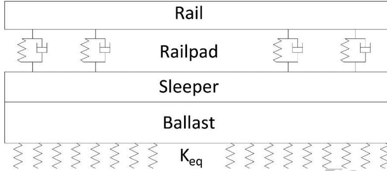
Figure 1: Ballasted track model structure
