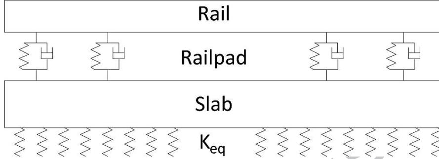
Figure 2: Slab track model structure
