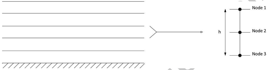
Figure 4: Discretization into thin layers with quadratic interpolation
