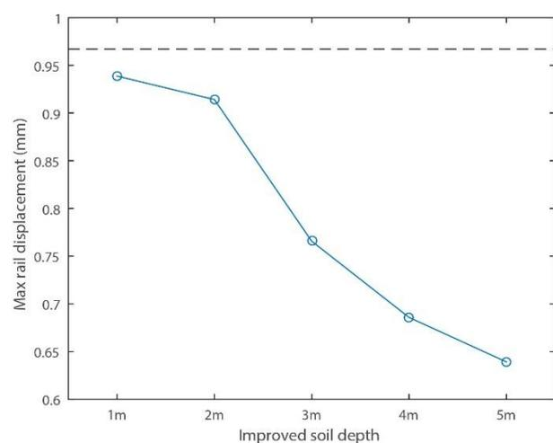
Figure 22: Maximum downward rail displacement for Soil 3. (Left) Ballasted track; (Right) Slab track; Dashed black line represents the original value
