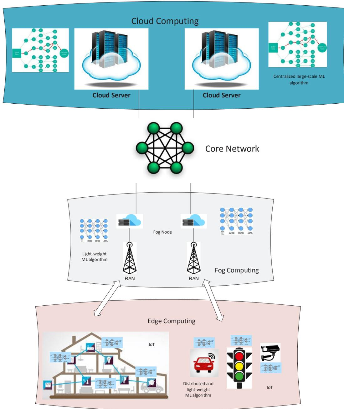
Fig. 4. Distributed and light-weight ML algorithms in 5G.
