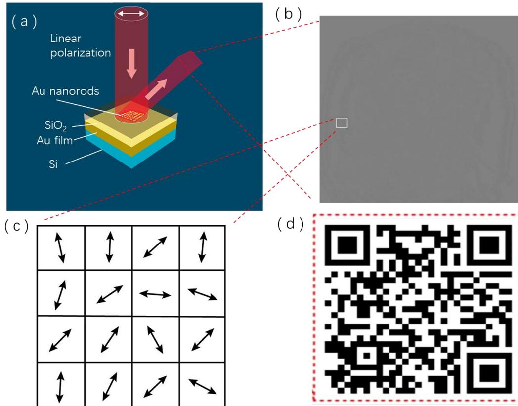
Figure 1 Schematic of the mechanism to hide a QR code in a laser beam. (a) Schematic of the design. (b) Intensity profile. (c) Schematic of polarization distribution in the white square area in (b). (d) Target QR code.
