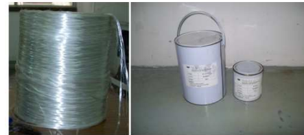
Figure2. E-600 woven roving fiber glass mixed with epoxy resin.
