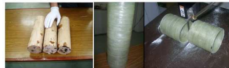
Figure3. Wooden mandrels and cutting process
