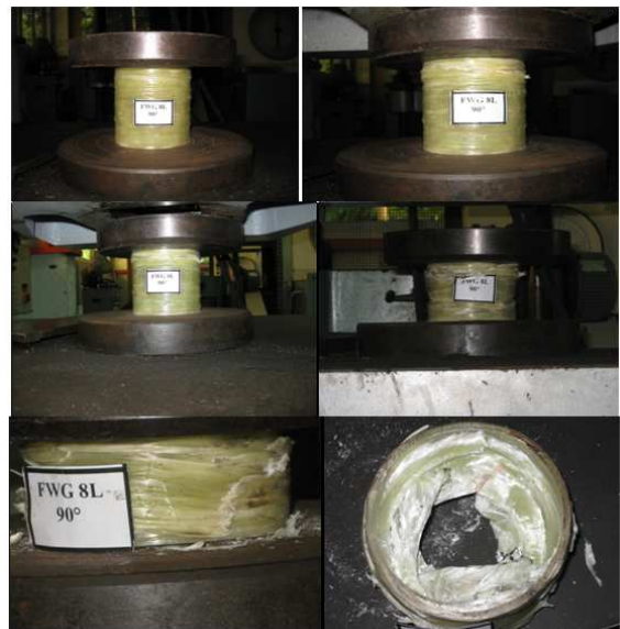
Figure8. Progress of Crashing FWG-8L-90°
