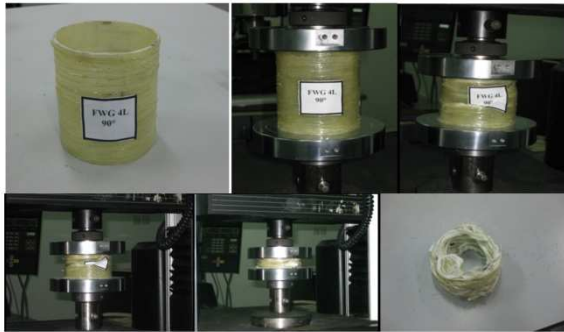
Figure6. Progress of Crashing FWG-4L-90°
