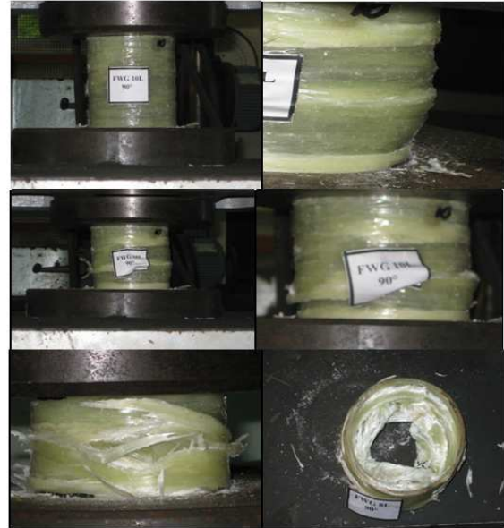
Figure9. Progress of Crashing FWG-10L-90°
