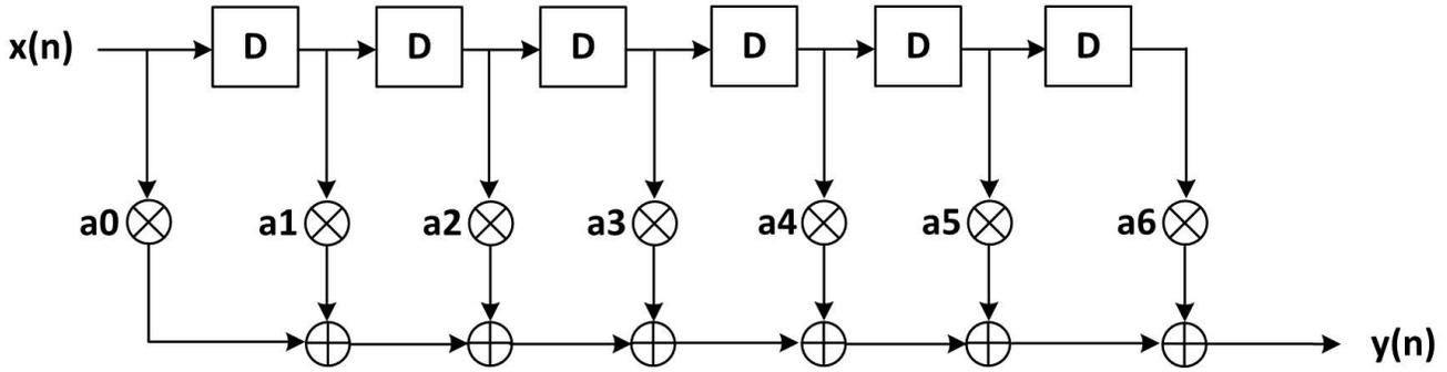
Figure 3: Structure of the SC 6th-order FIR filter.
