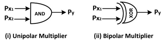
Figure 1: Stochastic Multiplier for (i) SC-unipolar and (ii) SC-bipolar formats.
