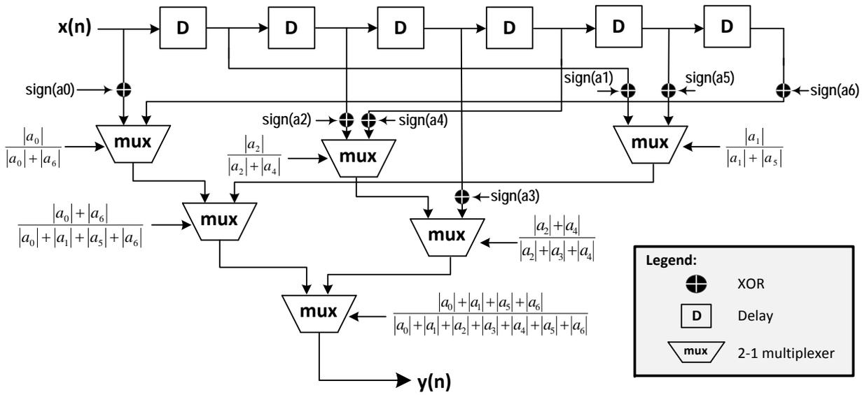
Figure 4: The circuit implementation of the 6th order SC FIR filter.
