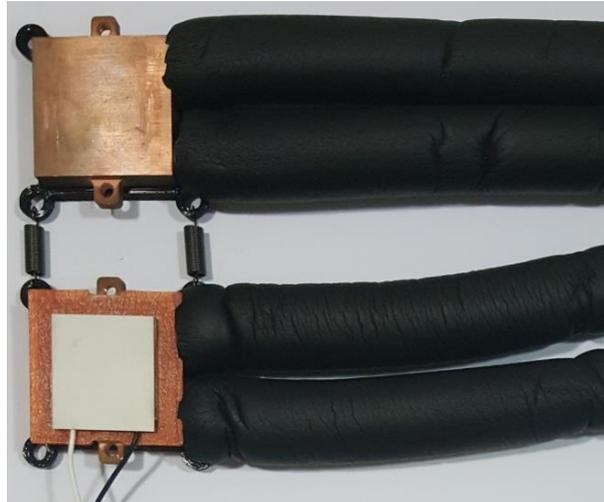
Figure 6 the TEG installed on one side of the water blocks.
