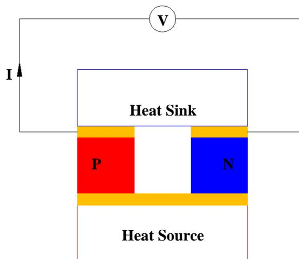
Figure 1 schematic diagram of a typical TEG.
