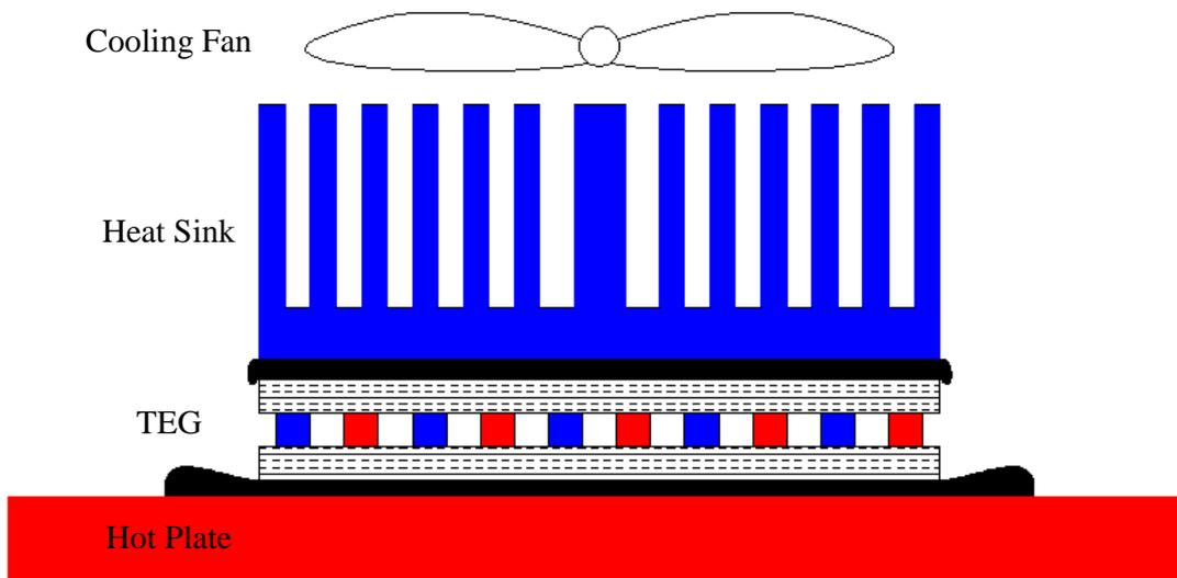
Figure 3 schematic diagram of the experimental setup.
