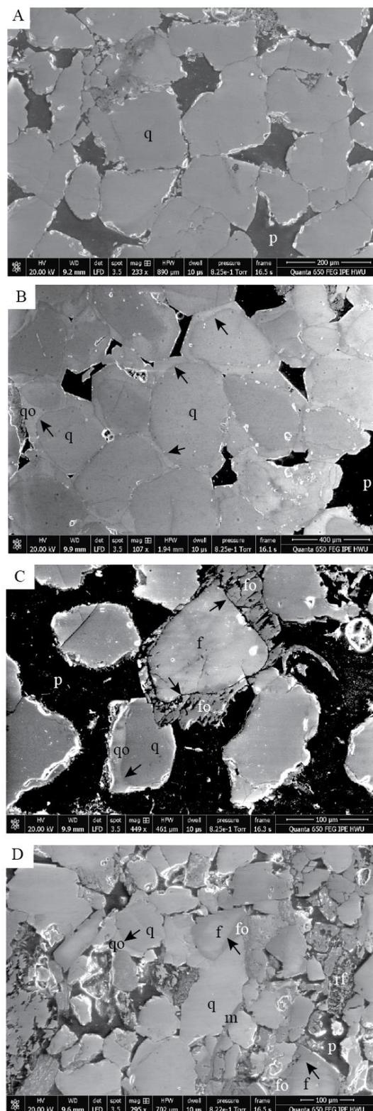
**Figure 4** Gaseous secondary electron (GSE) images. A= Darney sandstone, B= Lazonby sandstone, C= Locharbriggs sandstone and D= Red St. Bees sandstone. Key: p = pore, q = quartz, qo = quartz overgrowth, f = feldspar, fo = feldspar overgrowth, c = clay, m = mica
