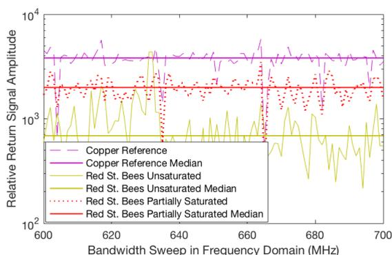
FIGURE 13 Return signal amplitudes for room-dry and partially saturated Red St. Bees sandstone, with copper sheet acting as an ideal reflector, and with data medians indicated over a 100 MHz sample size (between 600-700 MHz bandwidth sweep, see Figure 12)
