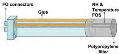
Figure 3 (above): Schematic of a fibre-optic humidity sensor.
