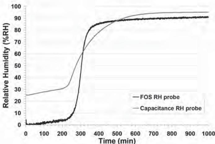
Figure 4 (left): Comparison of RH values between fibre-optic RH sensor and commercial capacitance-based RH sensor in a capillary absorption test.
