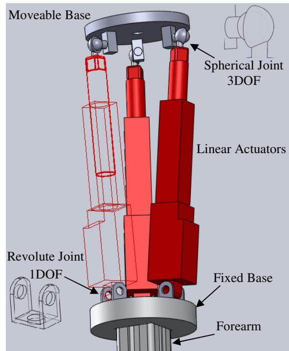
Figure 2. Robotic arm wrist (CAD Model)
