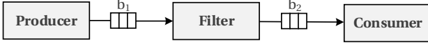
(a) An example of a dataflow network with three actors (i.e. Producer , Filter and Consumer ) and two buffers (i.e. b_1 and b_2 ).
