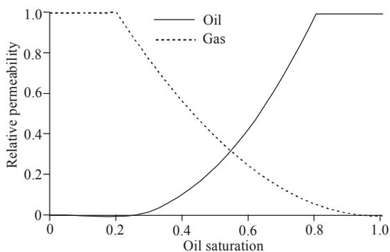
Fig. 2: Relative permeability curves vs. oil saturation
