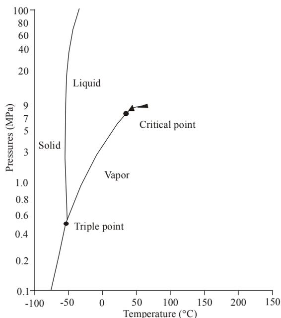
Fig. 1: CO<sub>2</sub> phase diagram (Baviere, 1980)
