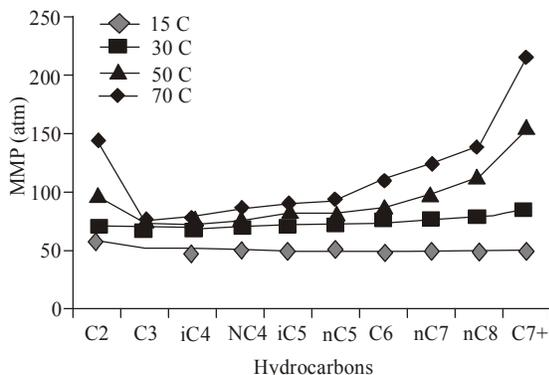
Fig. 5: MMP of pure hydrocarbons in different temperature
