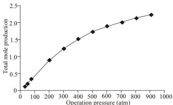
Fig. 4: Methane slimtube simulation results in T = 50 °C
