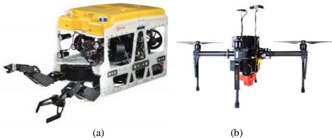
Fig. 1. (a) Inspection ROV for subsea oil and gas assets ( http://www.rov.org ) (b) Inspection drones for wind turbine nacelle components ( www.aerialmediascotland.co.uk ).
