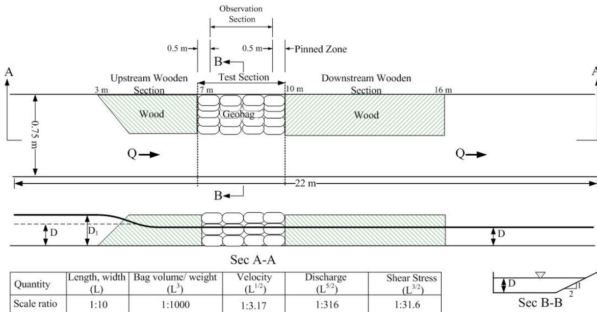
**Figure 2: Schematic of flume setup**
