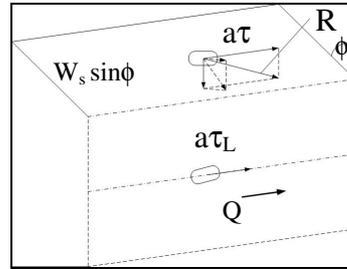
(b) Sediment particle resting on channel (Chow, 1959)
