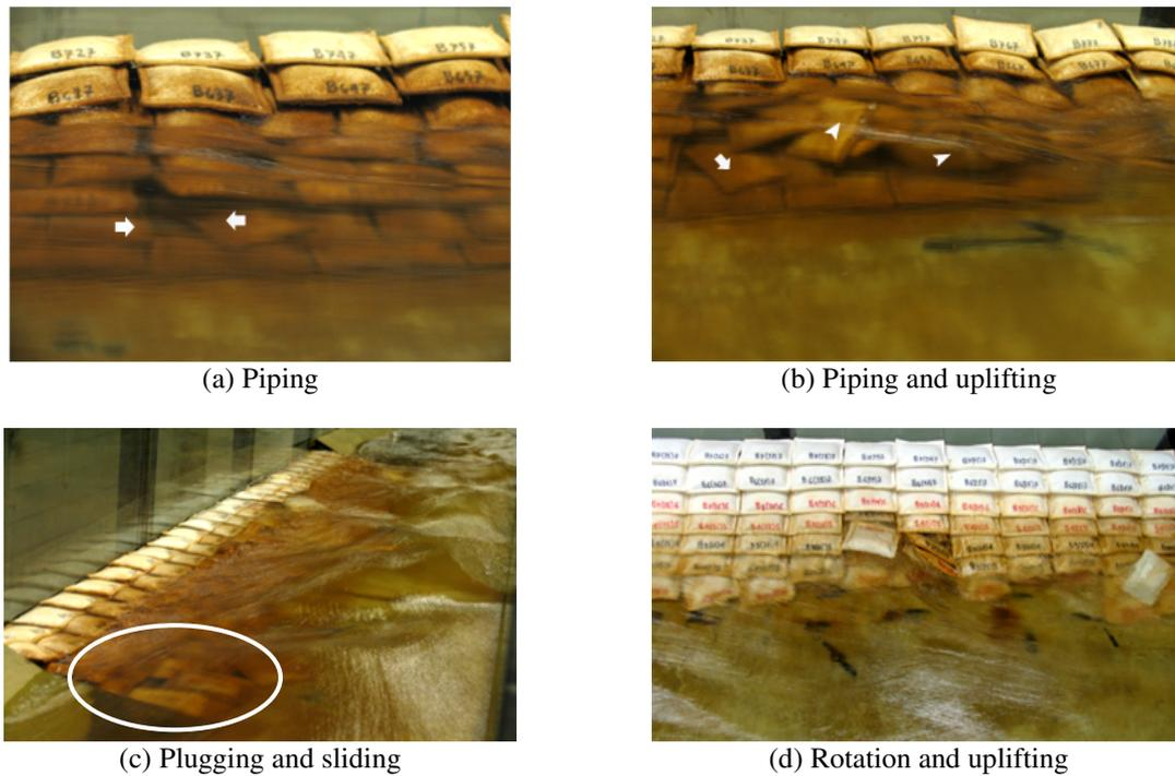
**Figure 3: Different failure modes observed in the physical model (a to d)**
