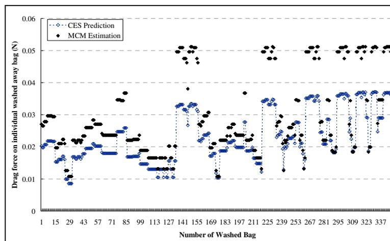
**Figure 5:** Estimation of the drag force on the washed away bag using MAM and CES
