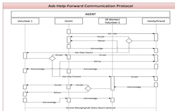
Fig. 2. Complex 3<sup>rd</sup> Party Ask-Help and Forward Communication Protocol in ER-ACL
