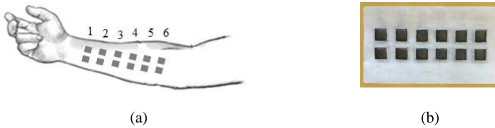
Figure 4. Electrode positions (a) Electrode positions on subject's forearm. (b) Assembled electrodes
