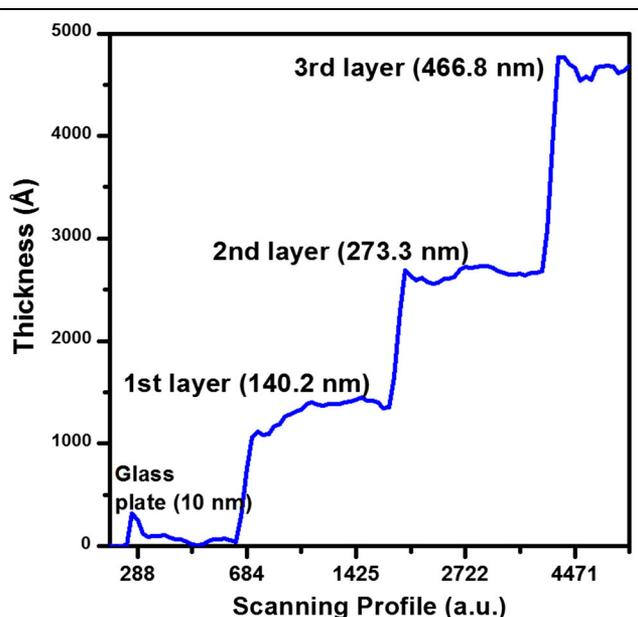
Fig. 1. Thickness measurement taken using a DEKTAK thickness profiler. The blue line indicates total structural thickness after each additional layer. The stacked layers were positioned off-axis to each other to specifically enable measurement.
