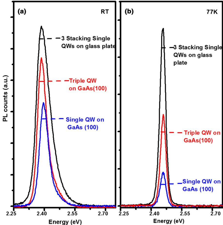
Fig. 2. PL spectra of single, triple QW and triple-stacked single QW at (a) 77 K and (b) RT. All measurements were taken under same conditions so a relative intensity comparison can be made.
