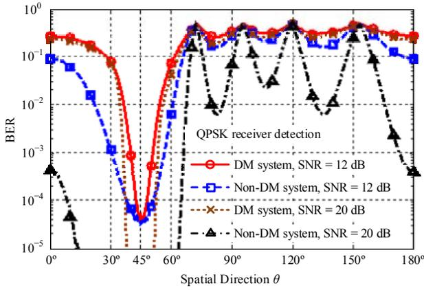
Fig. 4. Simulated BER spatial distributions in non-DM and single-beam dynamic DM systems with Gray-coded QPSK modulation for SNRs of 12 dB and 20 dB.
