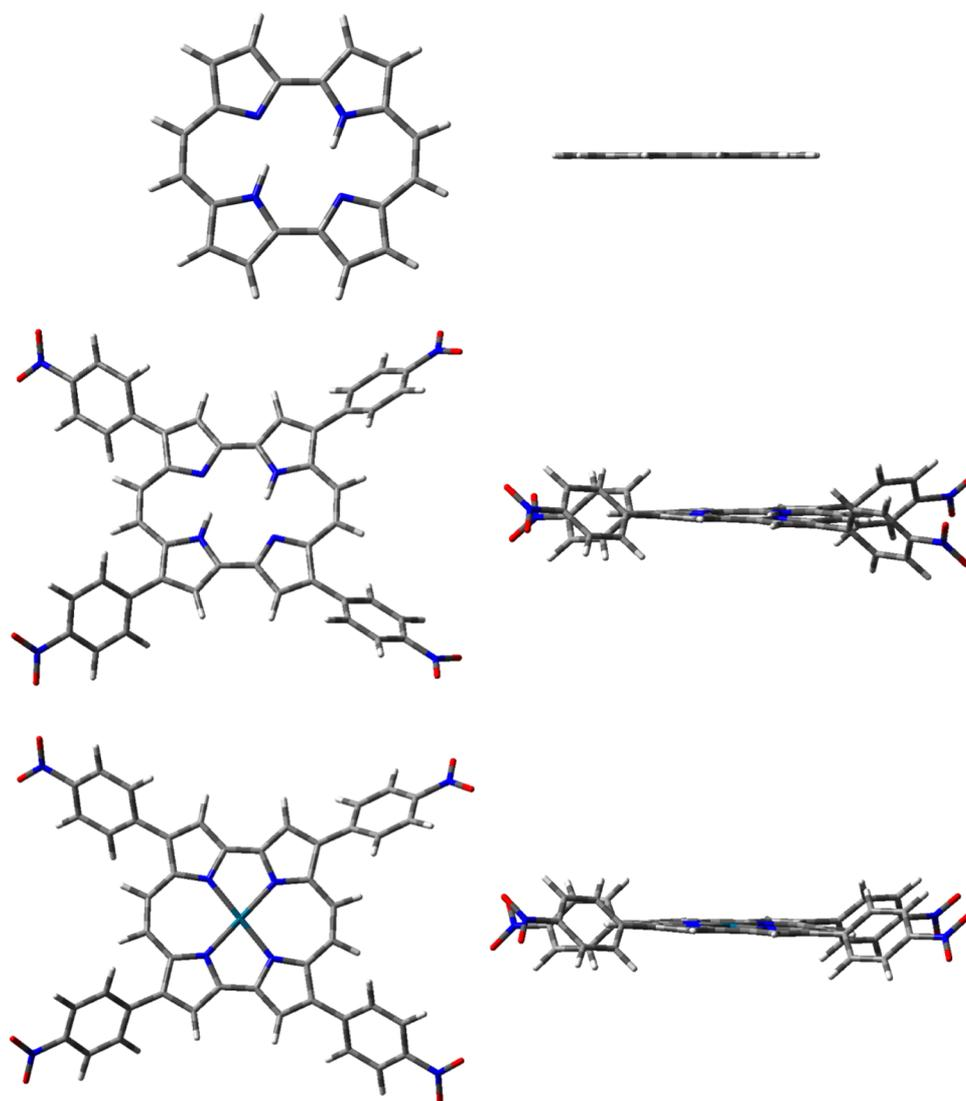
Figure 2. Optimized geometries of Pc, PcPN, and PdPcPN.
