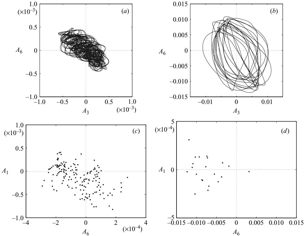
FIGURE 15. Phase portraits and Poincaré sections in the  $m=3$  regime: (a) phase portrait of the amplitude of  $A_6$  against  $A_3$  for  $Ta=2.0 \times 10^6$ , (b) phase portrait for  $Ta=3.25 \times 10^6$ ; (c) Poincaré section at  $A_3=0$  showing  $A_1$  against  $A_6$  for  $Ta=2.0 \times 10^6$ . (d) Poincaré section as (c) but for  $Ta=3.25 \times 10^6$ .
