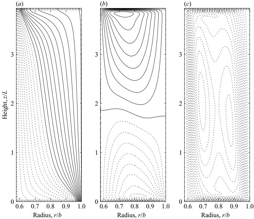
FIGURE 6. Zonal mean fields at  $Ta = 200\,000$  using air as the working fluid. (a) Temperature (contour interval = 0.1, normalized to an imposed temperature difference of  $\pm 1.0$ ), (b) zonal velocity  $V_\phi$  (contour interval = 0.25) and (c) meridional stream function (contour interval = 0.01). Dotted lines indicate negative values.
