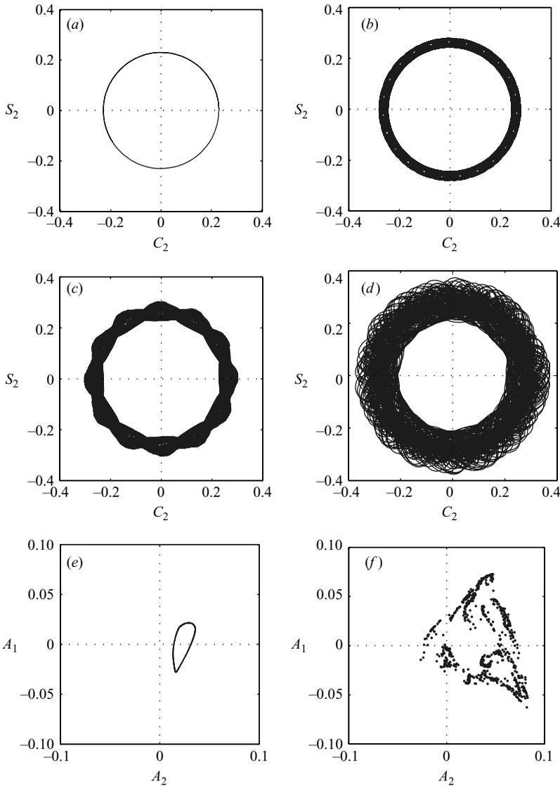
FIGURE 8. Phase-space representations of: (a) a steady 2S ( $Ta=200\,000$ ), (b) a 2AV ( $Ta=215\,000$ ), (c) a quasi-periodic 2MAV ( $Ta=220\,000$ ), and (d) a chaotic 2MAV ( $Ta=229\,250$ ). The phase-space diagrams show the time series of the sine component against that of the cosine component of mode  $m=2$ . (e, f) Poincaré sections of the amplitudes of  $m=1$  against  $m=2$  where  $m=4$  is zero, after the mean amplitudes had been subtracted.
