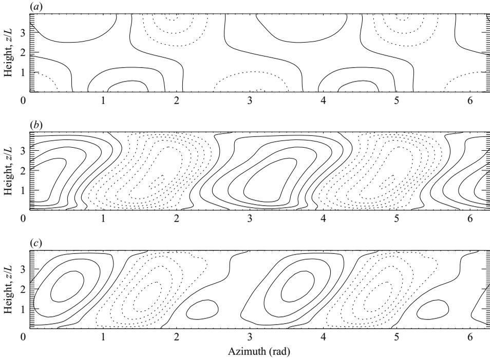
FIGURE 7. Azimuth–height maps of eddy fields (with azimuthal flow removed) in a typical simulation of a 2S flow at  $Ta = 200\,000$  using air as the working fluid. (a) Pressure (contour interval = 0.05 dimensionless units), (b) temperature  $T'$  (contour interval = 0.05, normalised to an imposed temperature difference of  $\pm 1.0$ ) and (c) Vertical velocity (contour interval = 0.1 dimensionless units).
