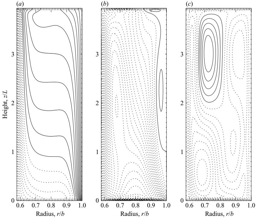
FIGURE 12. Zonal mean fields for the typical wave-3 simulation at  $Ta = 1.5 \times 10^6$  using air as the working fluid. (a) temperature (contour interval = 0.1, normalized to an imposed temperature difference of  $\pm 1.0$ ), (b) zonal velocity  $V_\phi$  (contour interval = 0.25 dimensionless units) and (c) meridional stream function (contour interval = 0.01 dimensionless units).
