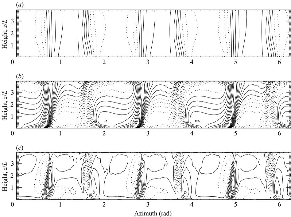
FIGURE 11. Azimuth-height maps of eddy fields (with azimuthal flow removed) in a typical simulation of the wave-3 flow at  $Ta = 1.5 \times 10^6$  using air as the working fluid. (a) Pressure (contour interval = 0.25 dimensionless units), (b) temperature  $T$  (contour interval = 0.05, normalized to an imposed temperature difference of  $\pm 1.0$ ) and (c) vertical velocity (contour interval = 0.5 dimensionless units).
