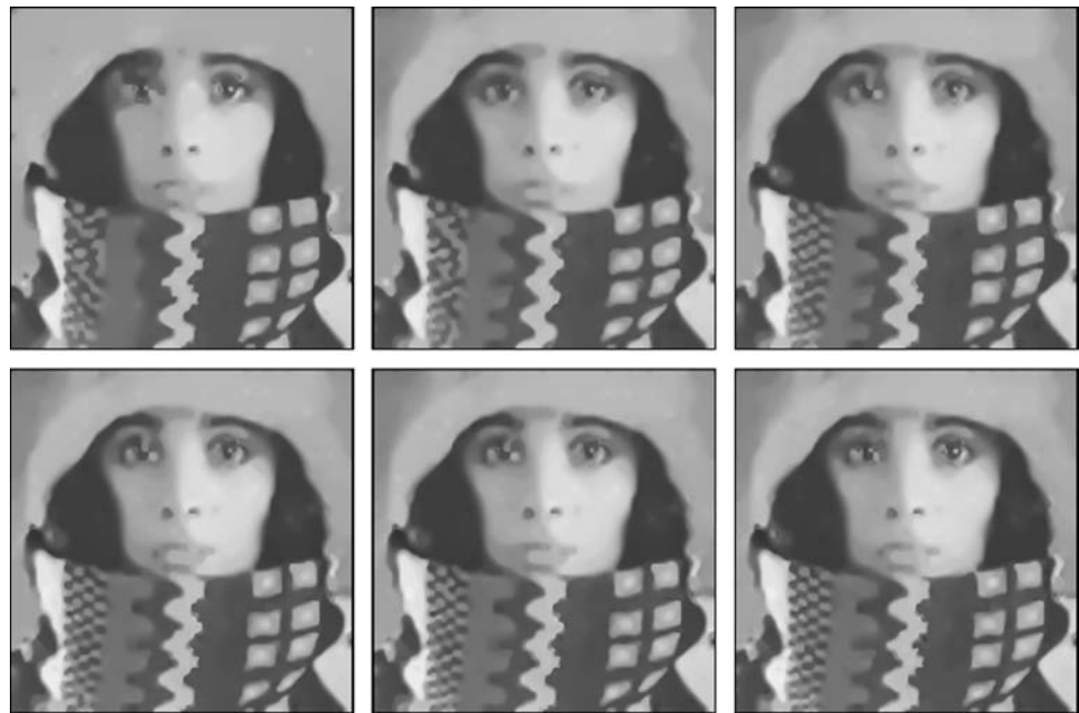
Fig. 6 Comparison of BTTC-based compression methods at a compression rate of 0.2 bpp. First row, left to right: EED-based decoding (Q64 + BTTC(L)-EED), with adaptive threshold (Q64 + BTTC(L,AT)-EED), with EED coding (Q64 + BTTC(EED,AT)-EED). Second row, left to right: with biasing (Q64 + BTTC(EED,AT) + B-EED), with post-quantisation to 64 grey levels (BTTC(EED,AT) + B + Q64-EED), with post-quantisation to 32 grey levels instead (BTTC(EED,AT) + B + Q32-EED)
