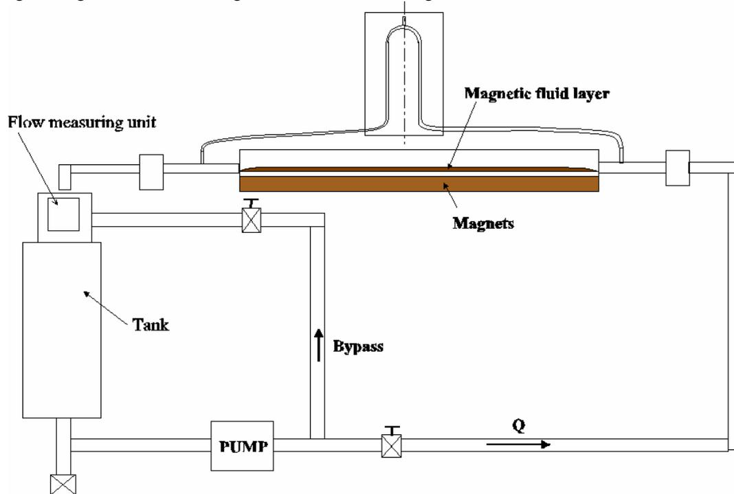
**Figure 1 Experimental rig**
