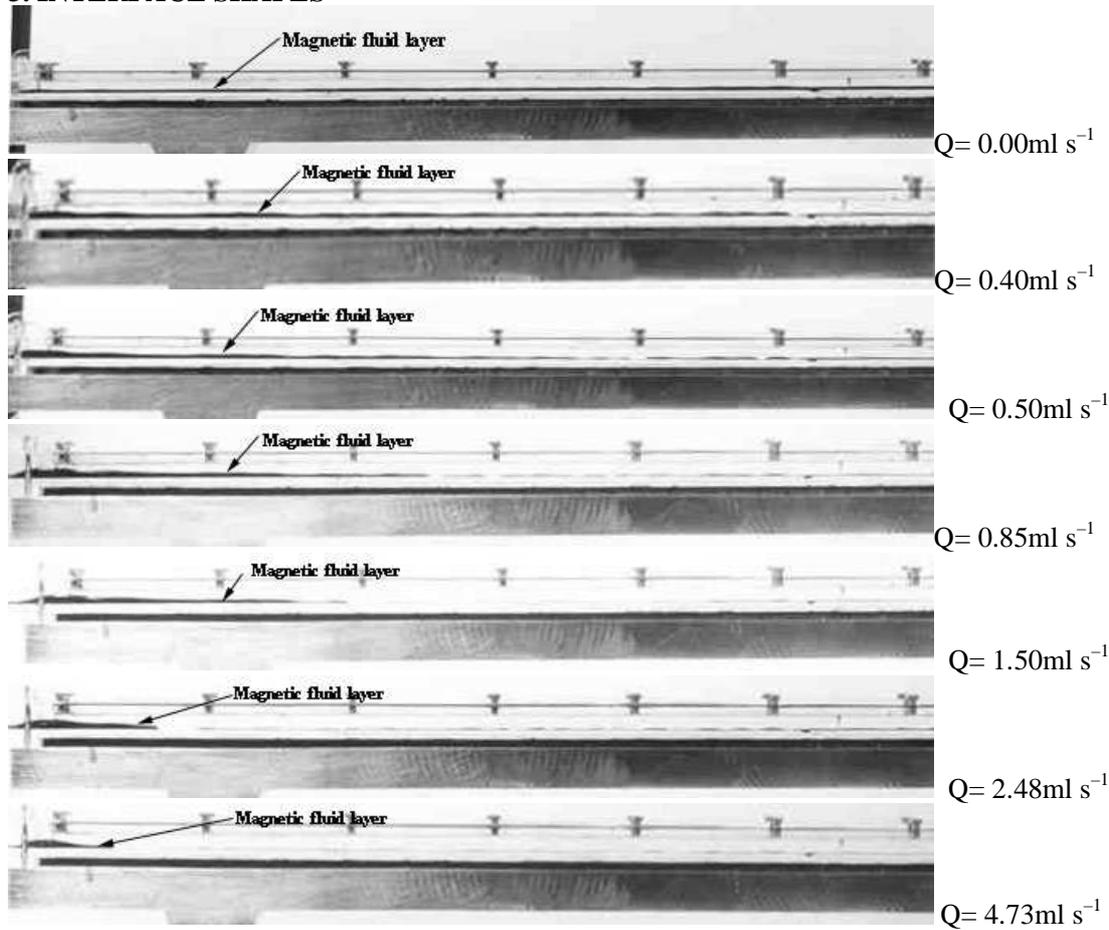
**Figure 3** Sample pictures of the magnetic fluid layer, magnet arrangement as in Figure 2 (a)
