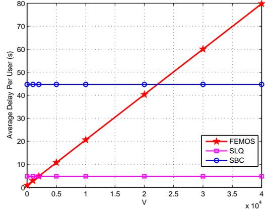
(b) Service Delay Per User vs. Parameter  $V$ .Fig. 4: Comparison of FEMOS and other FAN assignment schemes,  $A_{\max} = 100$  kbits,  $U = 100$ .
