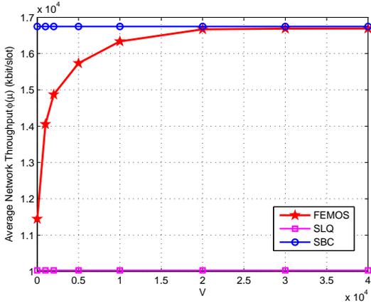
(a) Network Throughput vs. Parameter  $V$ .
