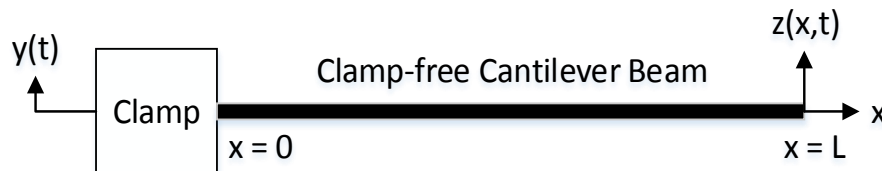
Figure 1. Cantilever beam under harmonic base excitation.
